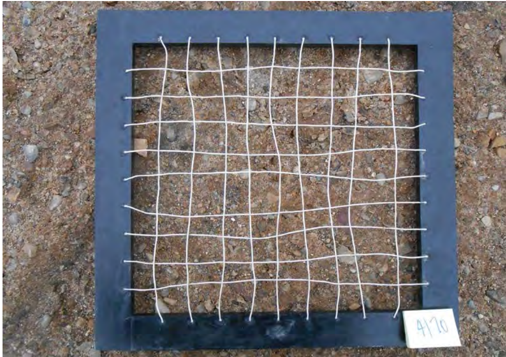
Variegated light brown-dark gray silty fine sand with some coarse gravel. Point 4170 was renumbered to 233 during construction due to the location of the point being outside ash boundaries.
