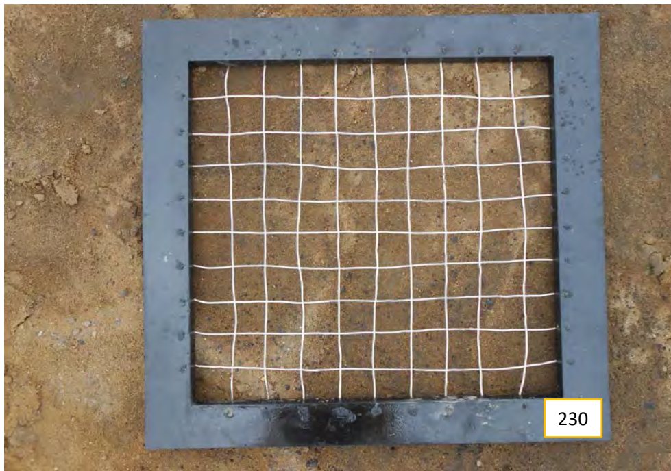
Brown silty fine sand with trace fine gravel
