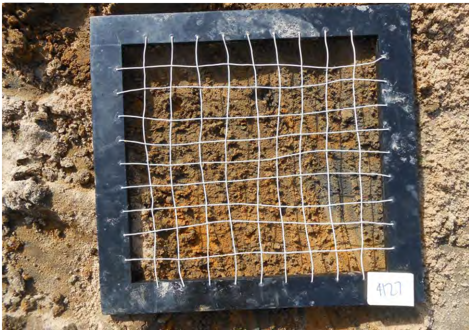
Brown silty fine sand with trace gravel
