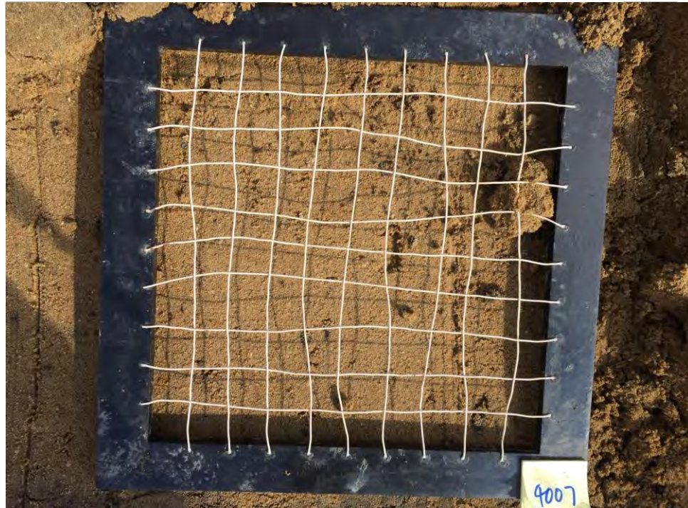
Brown silty fine sand with trace fine gravel
