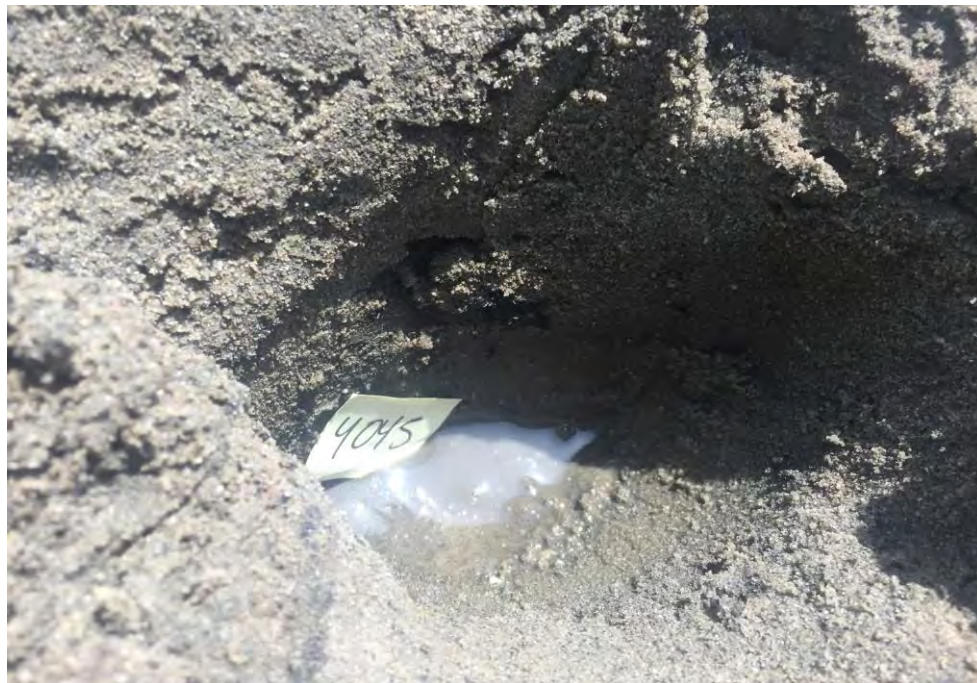
Brown silty fine sand with trace gravel
