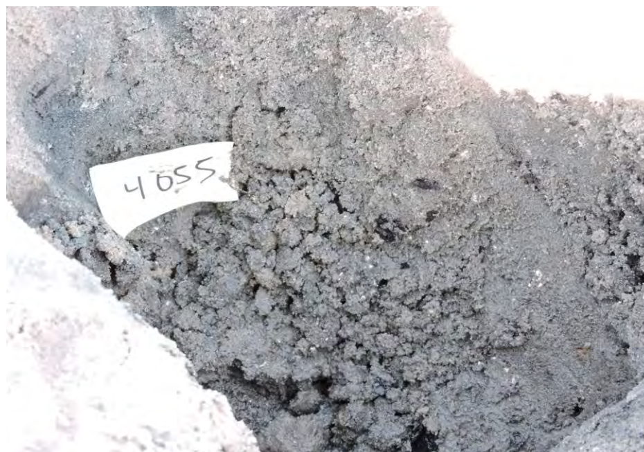
Medium brown silty fine sand with trace shells
