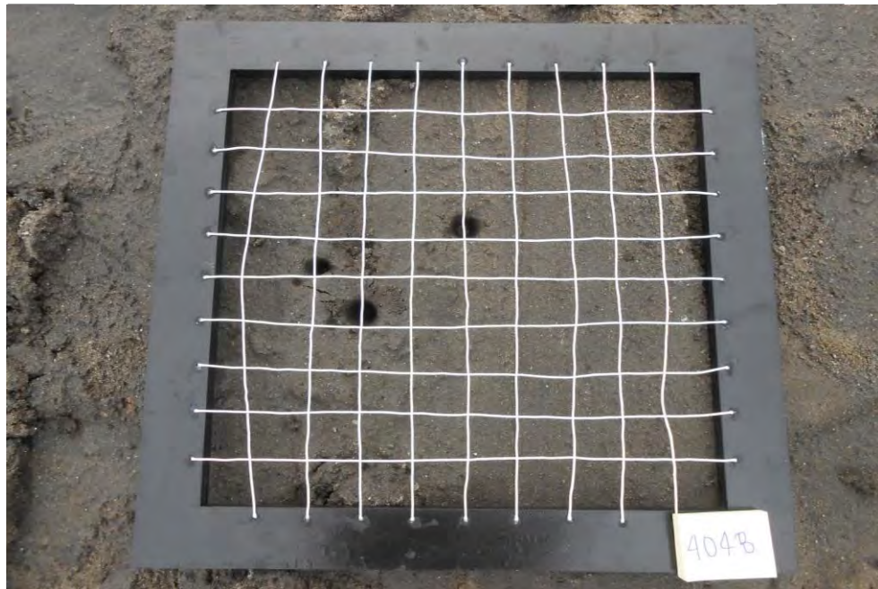
Dark gray silty fine sand with trace gravel and roots
