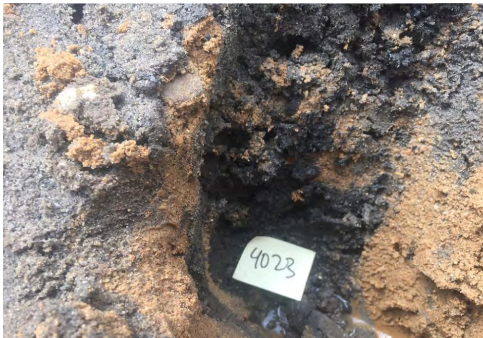
Gray silty fine sand with trace gravel
