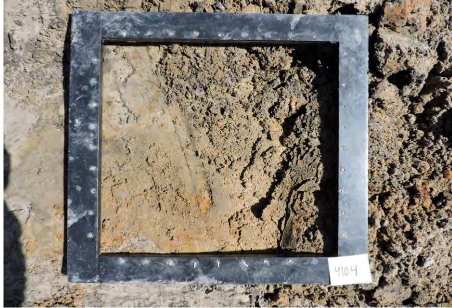
Brown-orange silty fine sand with peat layers
