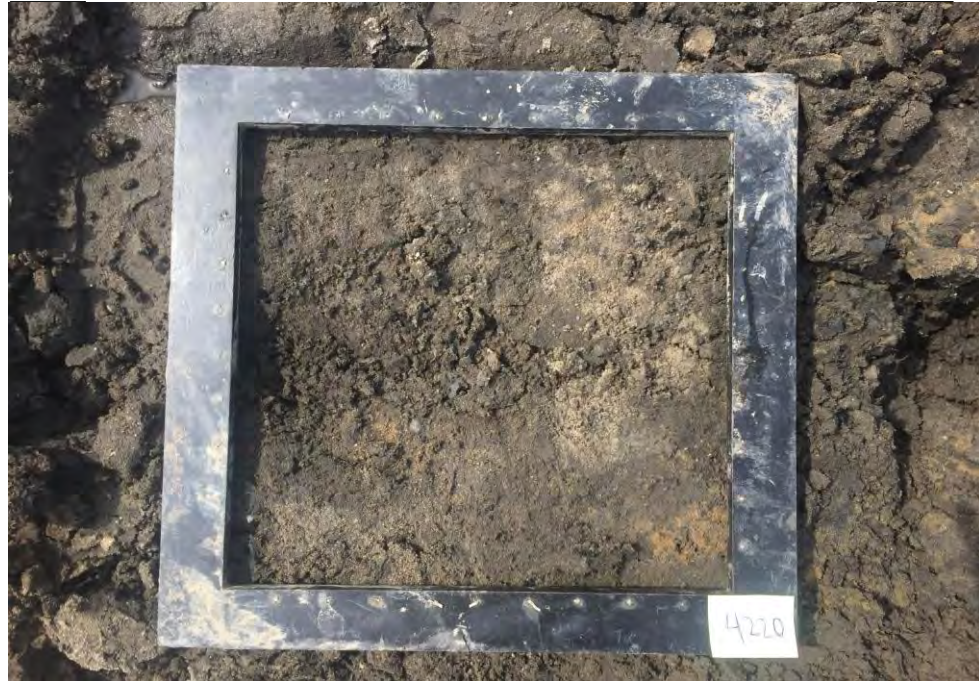
Brown silty fine sand with trace shells
