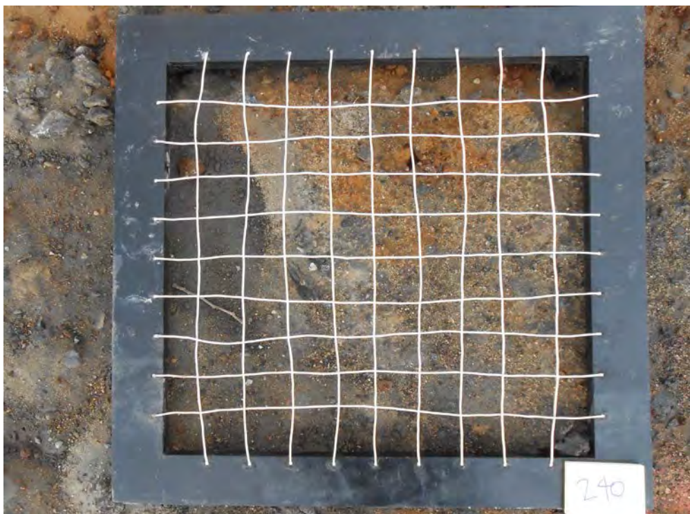
Variegated orange-gray silty fine sand with trace gravel
