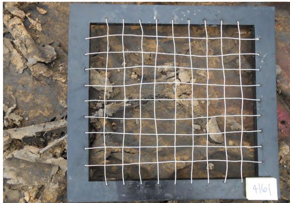
Variegated light brown-dark gray silty fine sand with trace roots
