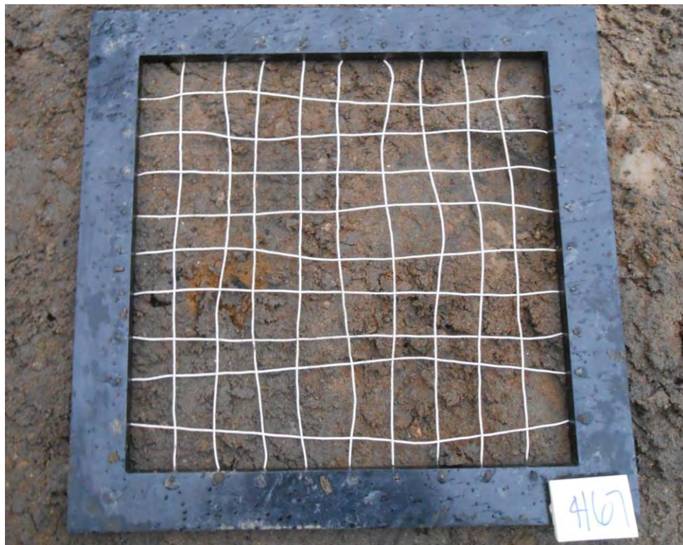
Variegated gray-brown silty fine sand with trace gravel
