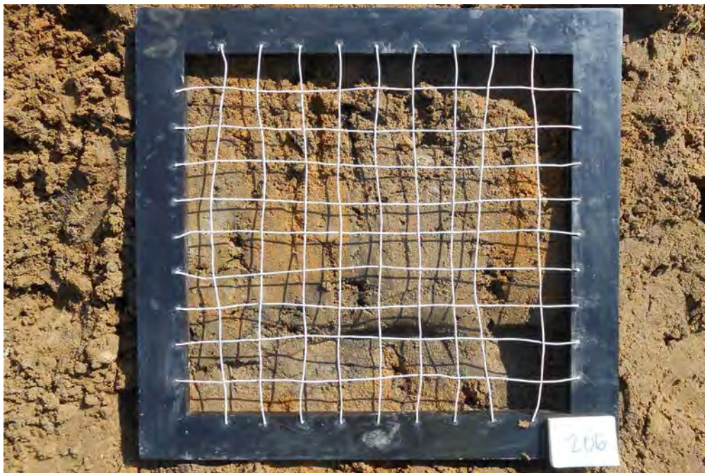
Brown silty fine sand with trace gravel and clay
