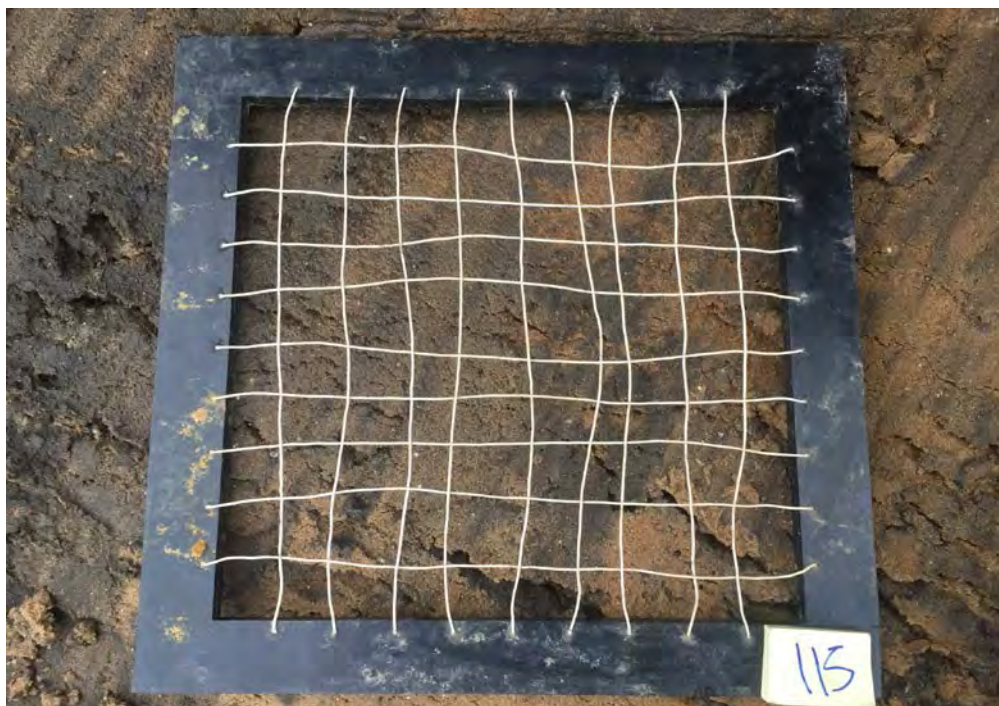
Variagated orange-brown silty fine sand with trace large sticks
