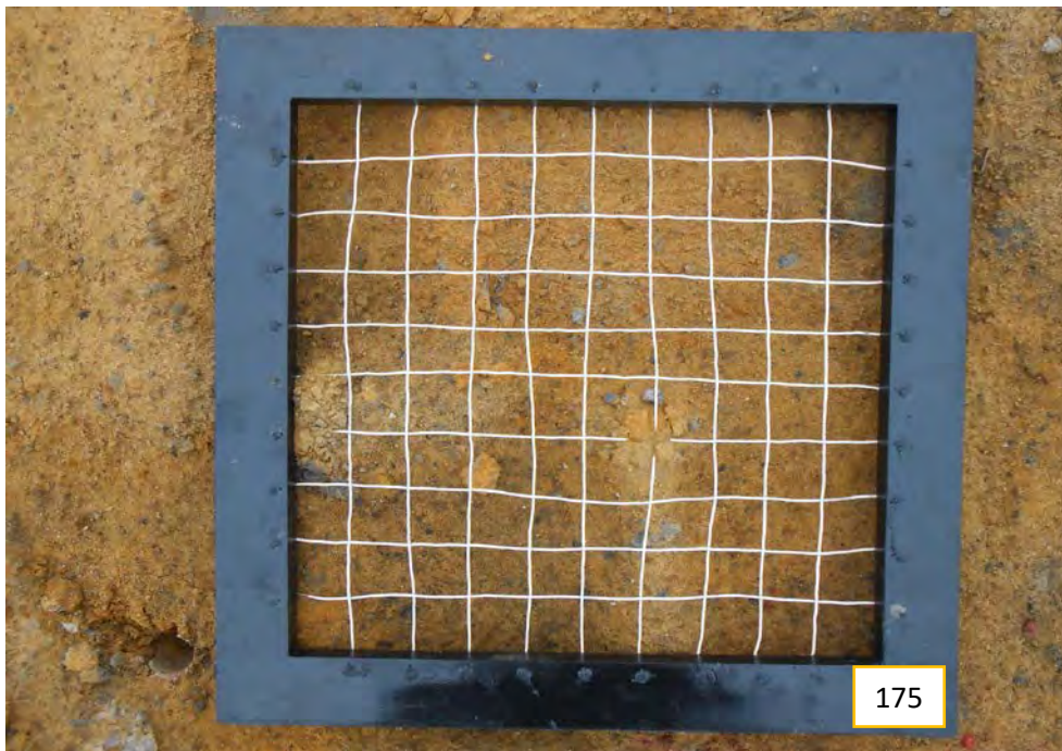
Orange silty fine sand with trace gravel
