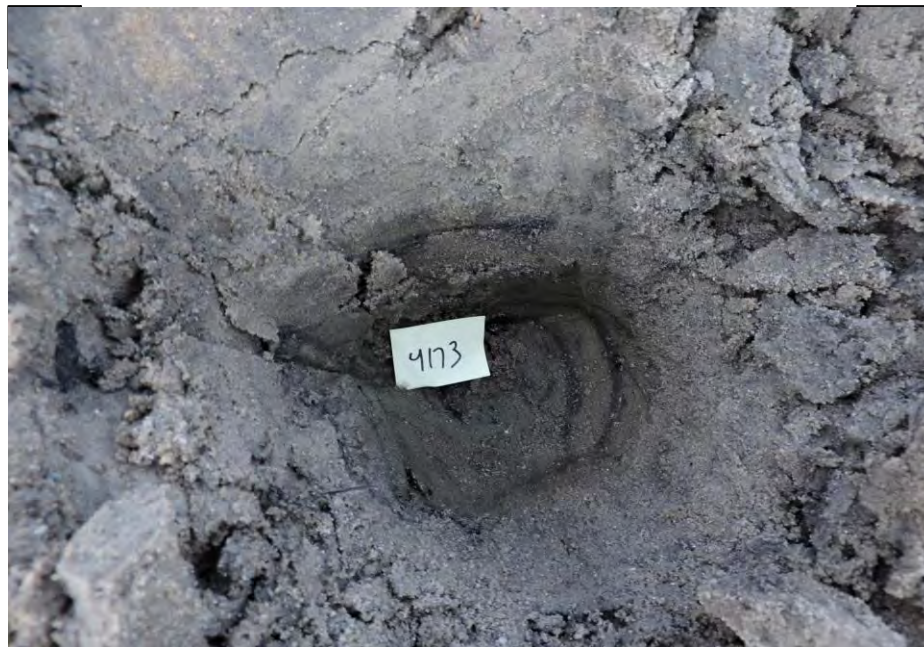
Dark brown silty fine sand with trace shells
