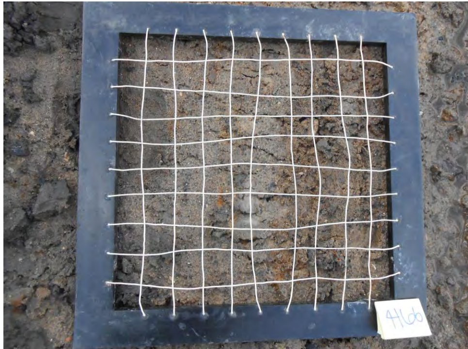
Variegated gray-brown silty fine sand with trace gravel
