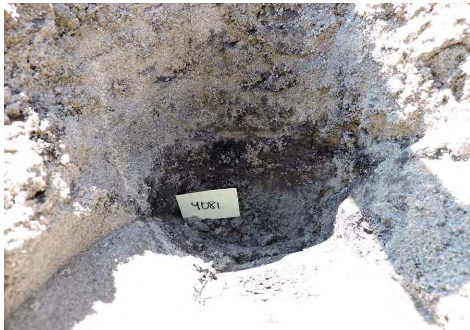
Light brown silty fine sand with trace peat and clay
