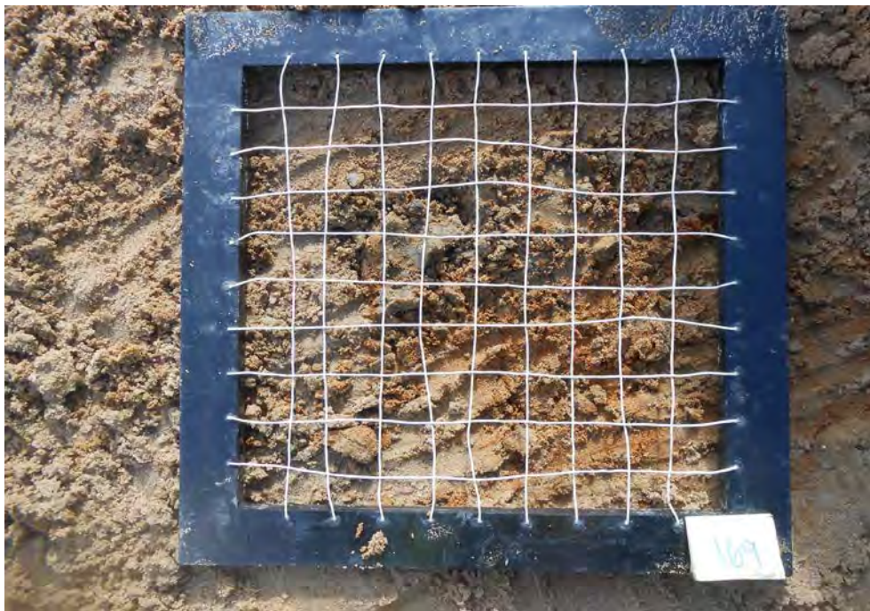
Brown silty fine sand with trace clay
