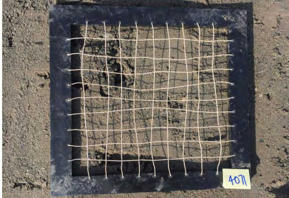
Light brown silty fine sand with trace gravel
