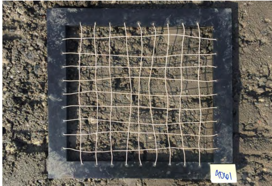
Gray silty fine sand with trace gravel and clay
