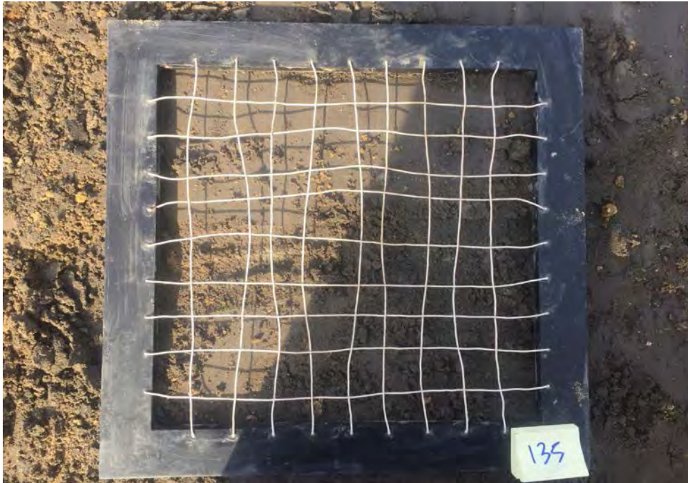
Light brown silty fine sand with trace gravel and roots
