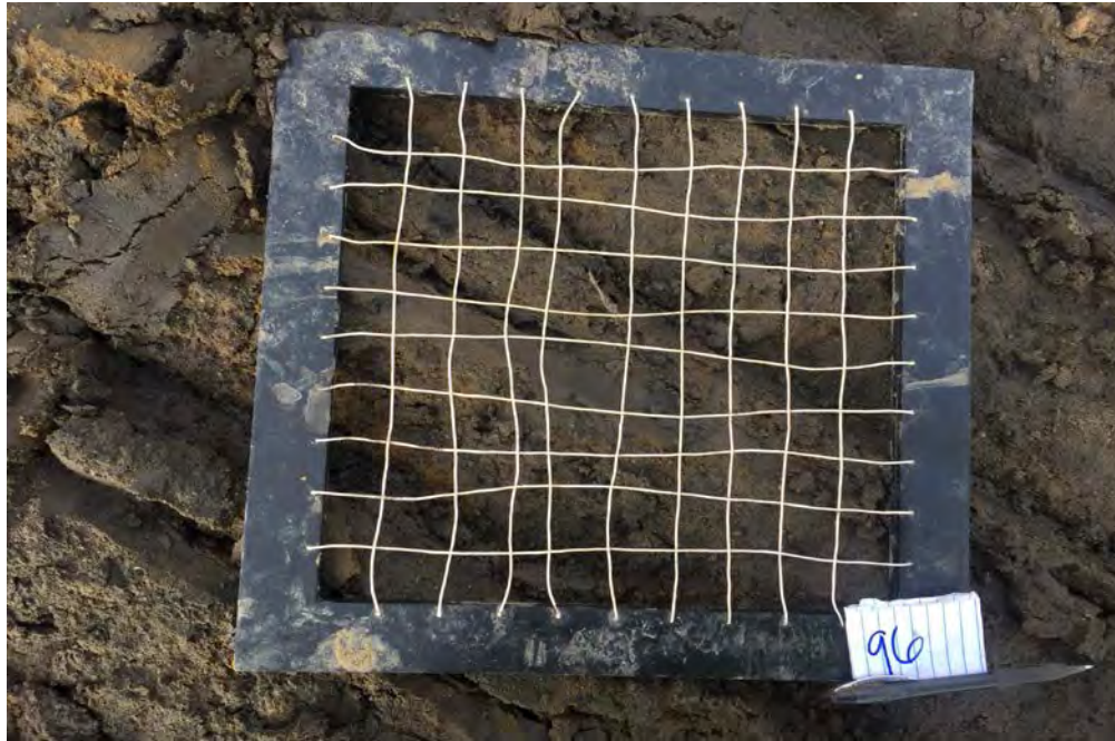
Variegated orange-gray silty fine sand with trace roots
