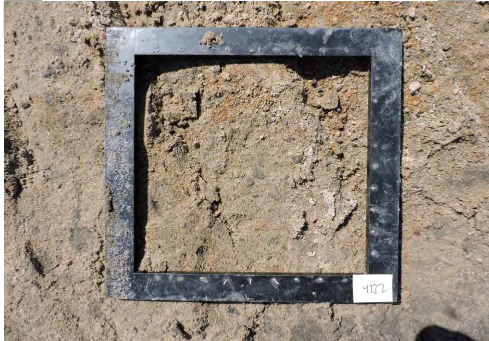
Brown silty fine sand with trace gravel
