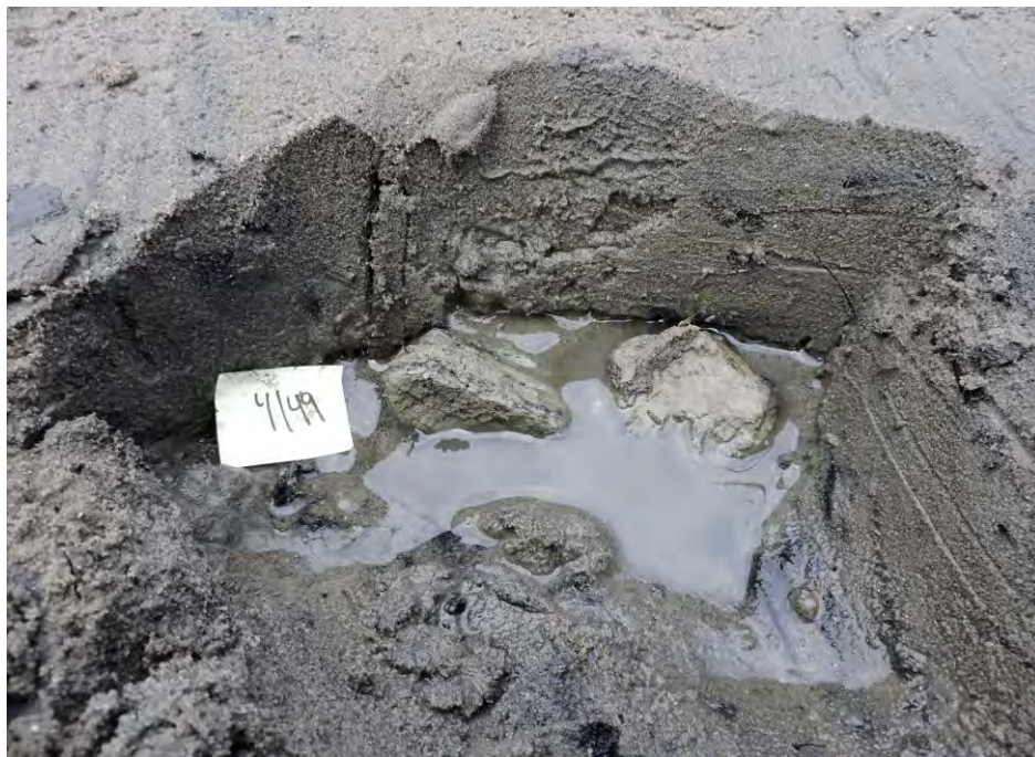
Dark gray silty fine sand with trace peat and trace clay
