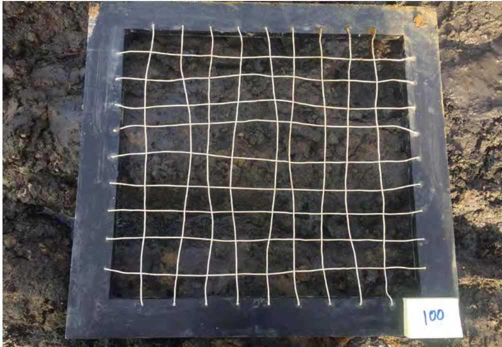
Medium gray silty fine sand with trace gravel and sticks
