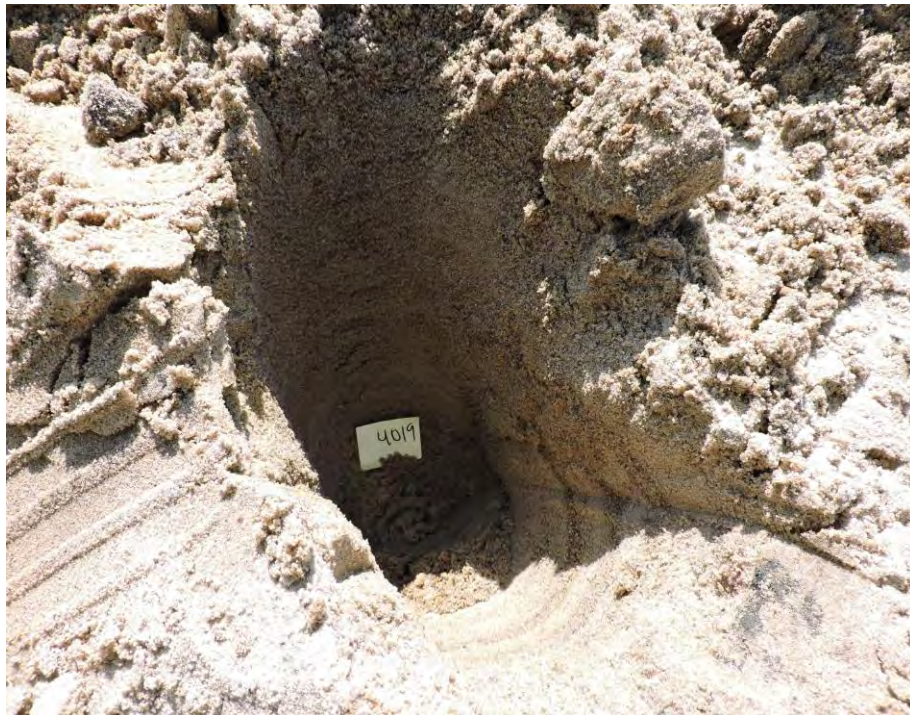
Brown-orange silty fine sand with trace gravel
