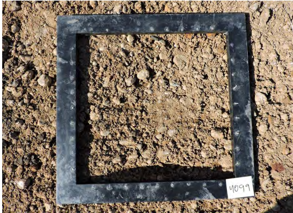
Light-dark brown silty fine sand with some medium gravel
