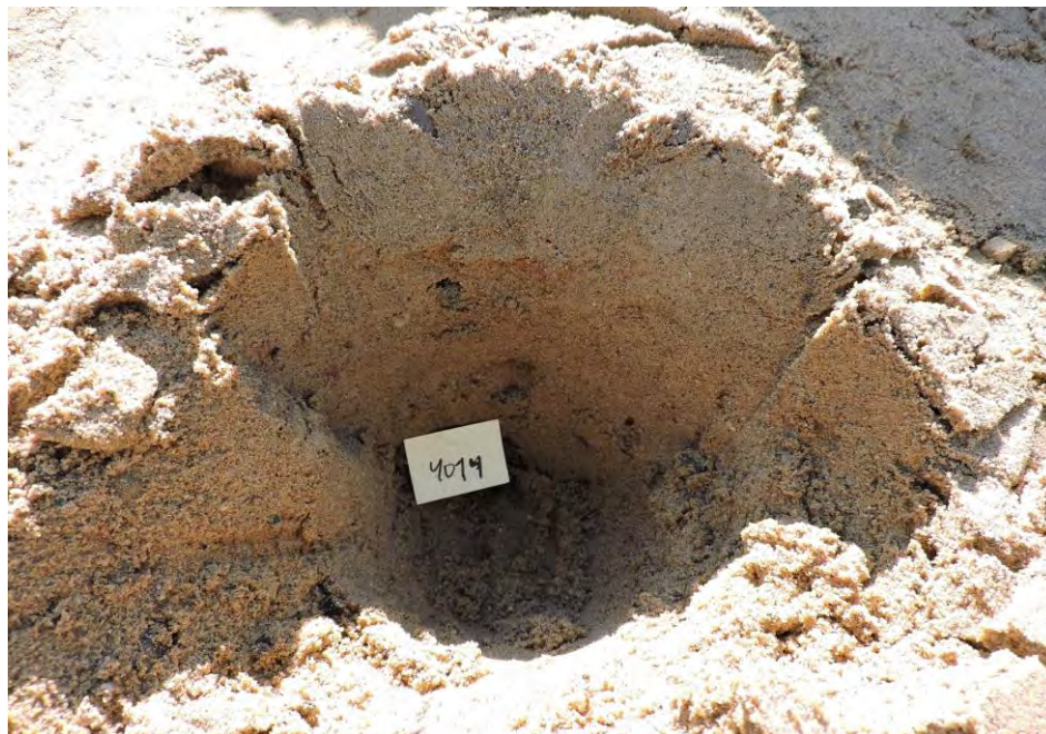
Medium brown silty fine sand with trace gravel
