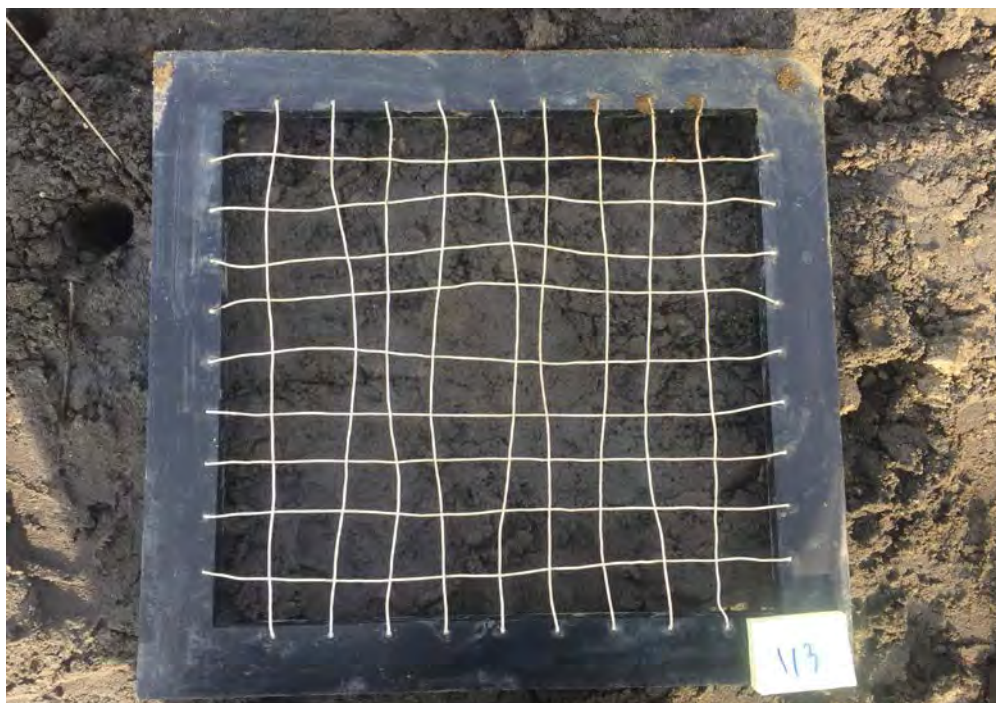
Dark brown silty fine sand with trace gravel and sticks
