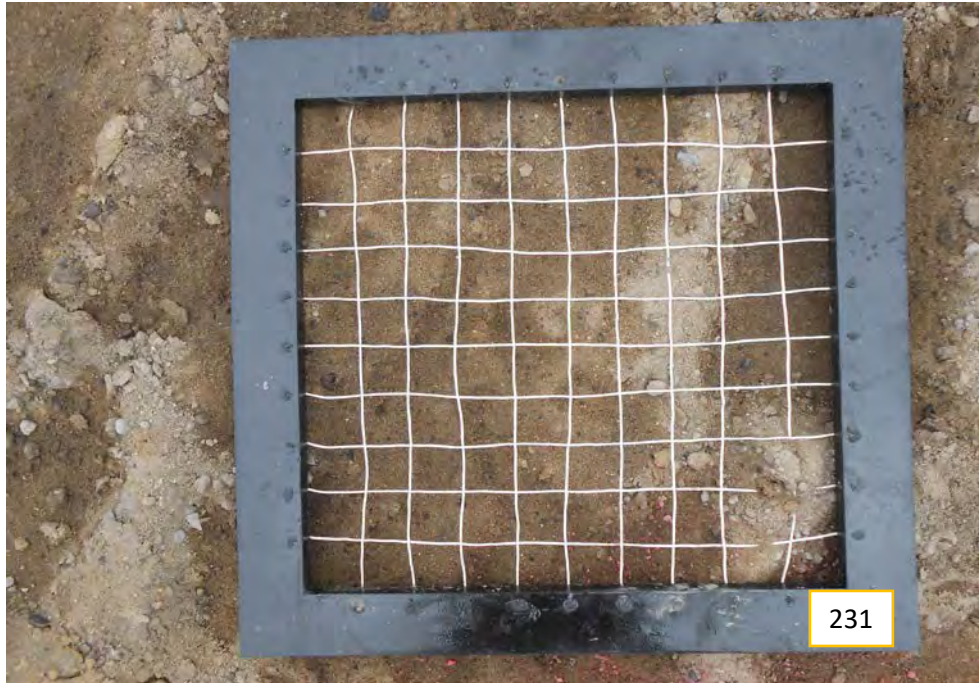
Brown silty fine sand with trace gravel
