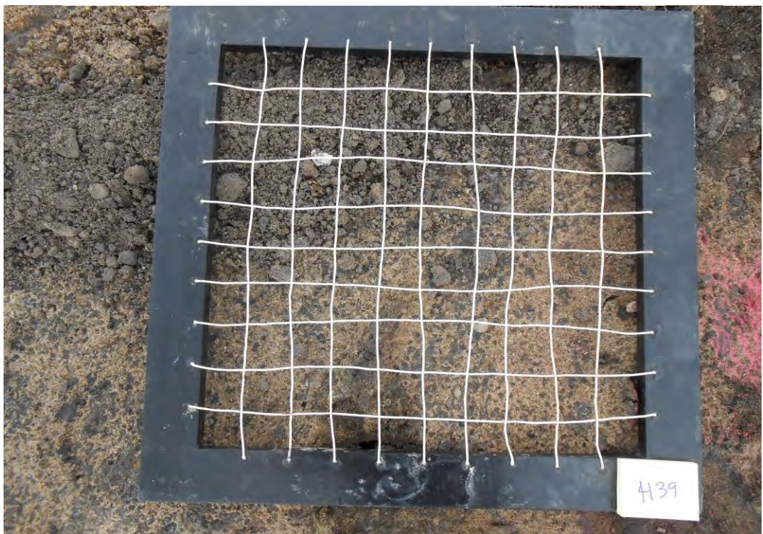
Variegated light gray-brown silty fine sand with trace gravel
