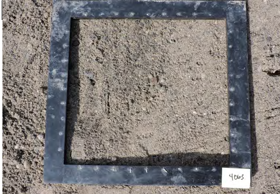
Light brown silty fine sand with some gravel
