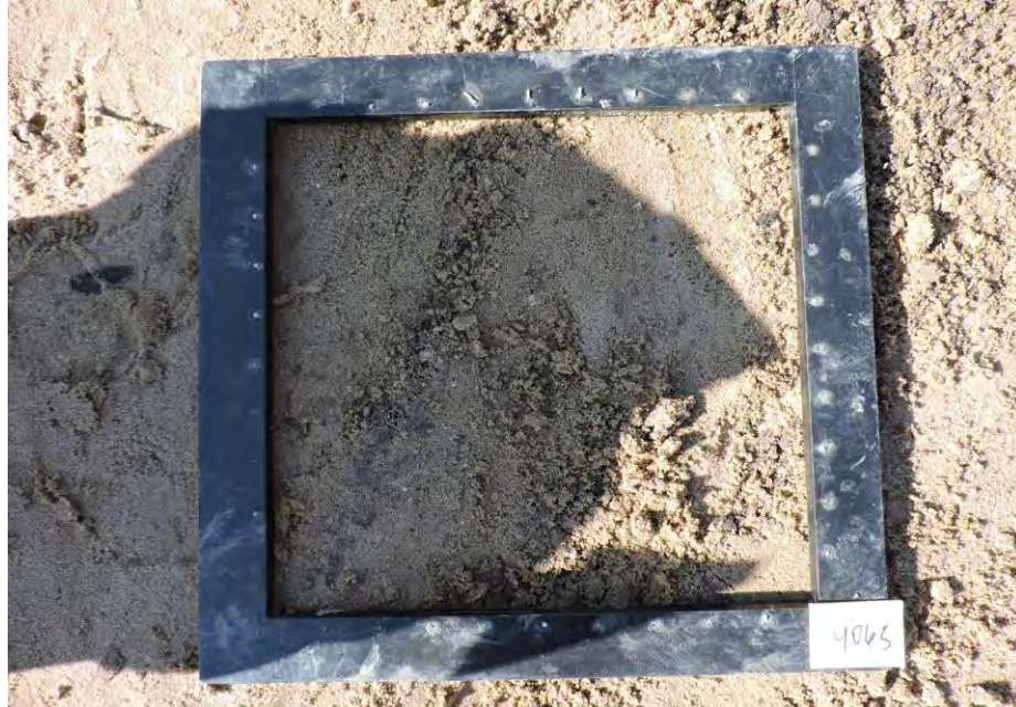
Light brown silty fine sand with trace gravel
