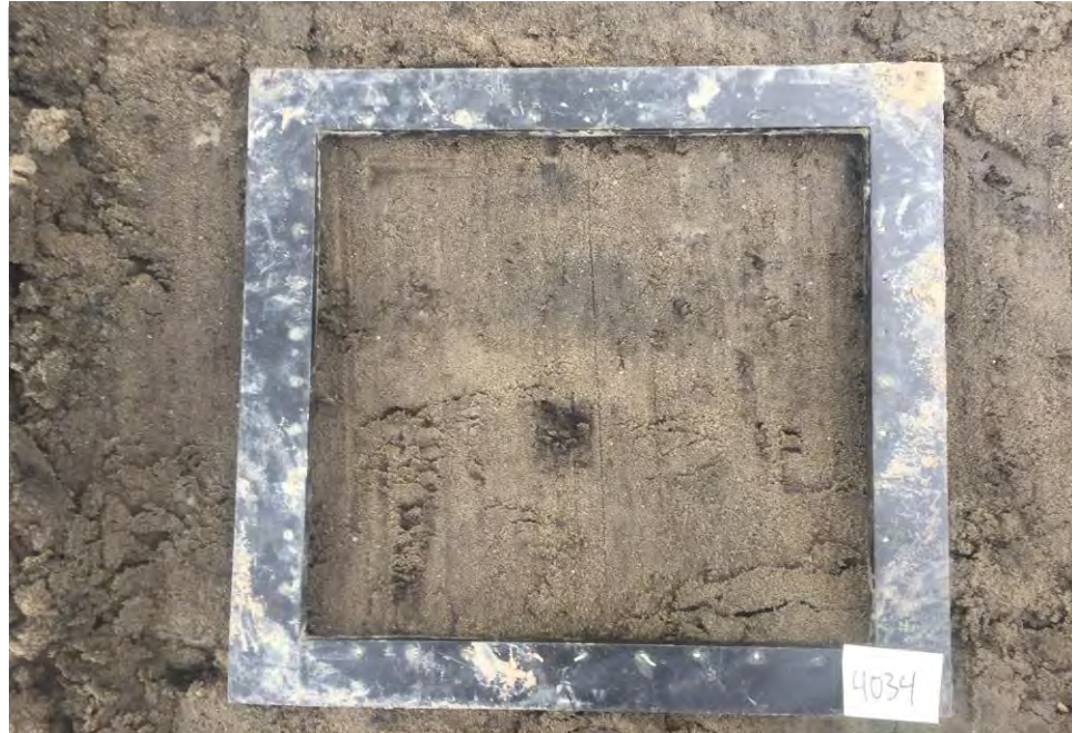
Brown silty fine sand with trace gravel
