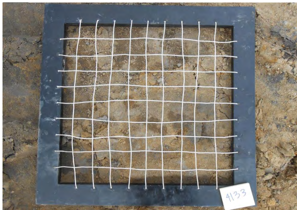
Gray silty fine sand with trace gravel
