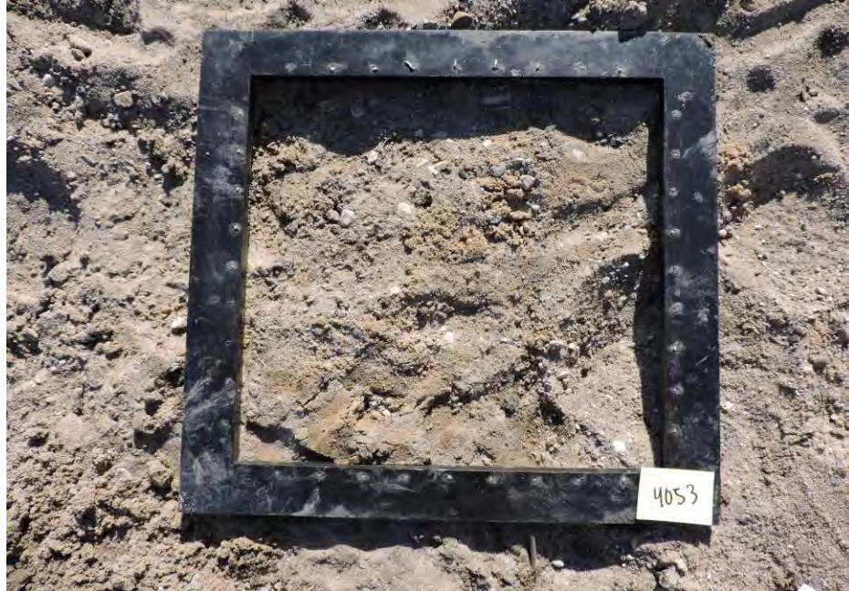
Light brown silty fine sand with little coarse gravel
