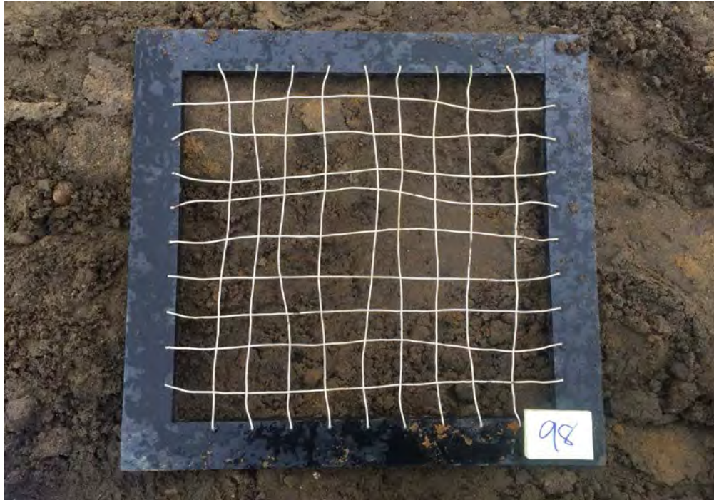
Variegated orange-brown silty fine sand with trace gravel
