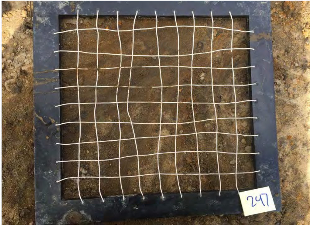
Brown silty fine sand with trace gravel
