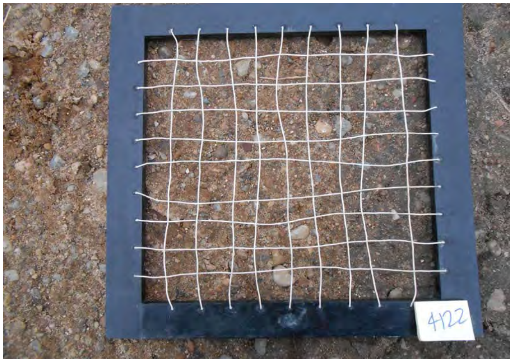
Variegated light brown-dark gray silty fine sand with some coarse gravel. Point 4122 was renumbered to 218 during construction due to the location of the point being outside ash boundaries.
