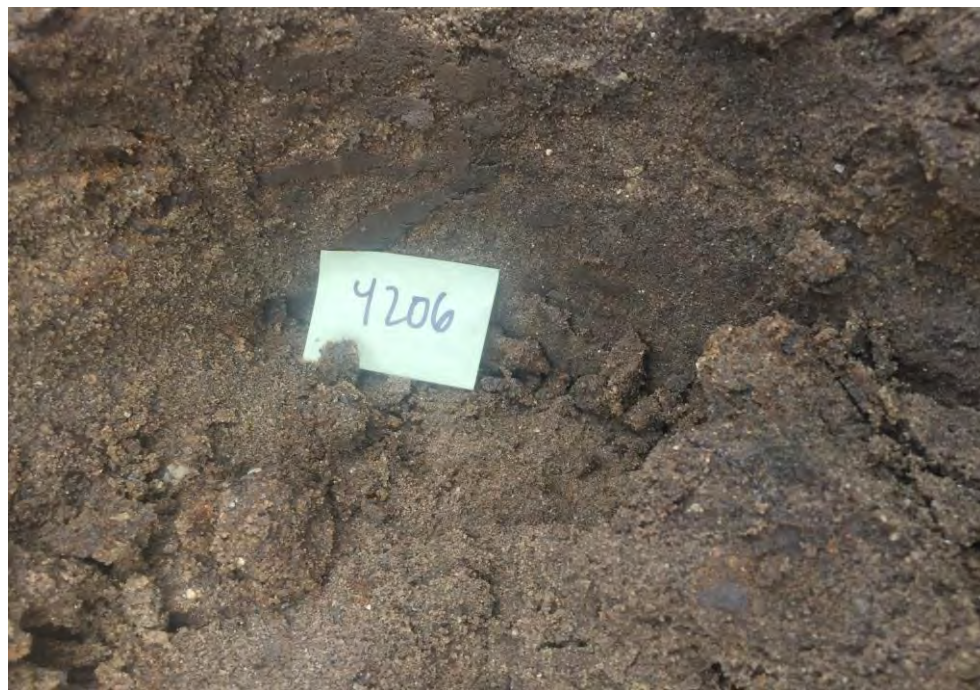
Brown silty fine sand with trace gravel
