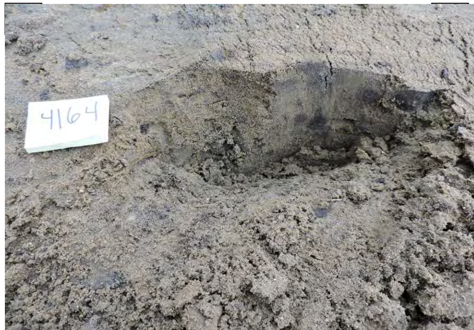
Brown silty fine sand with trace clay
