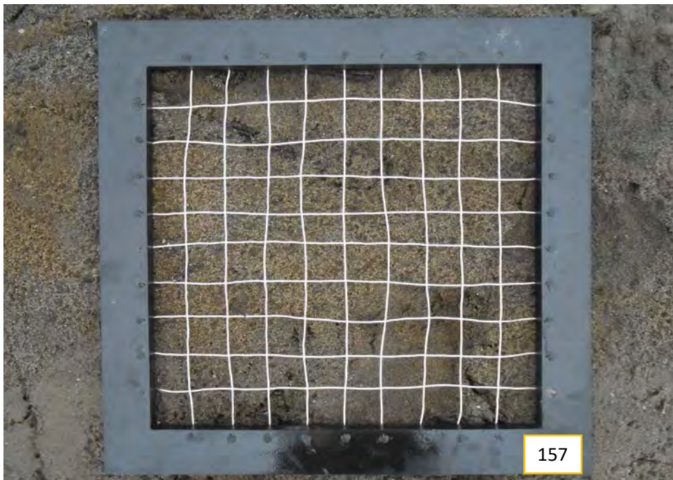
Variegated brown-gray silty fine sand with trace fine gravel
