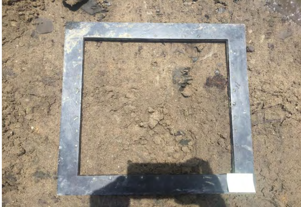
Brown silty fine sand with trace gravel
