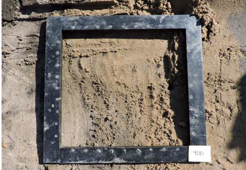
Light brown silty fine sand with trace peat and clay
