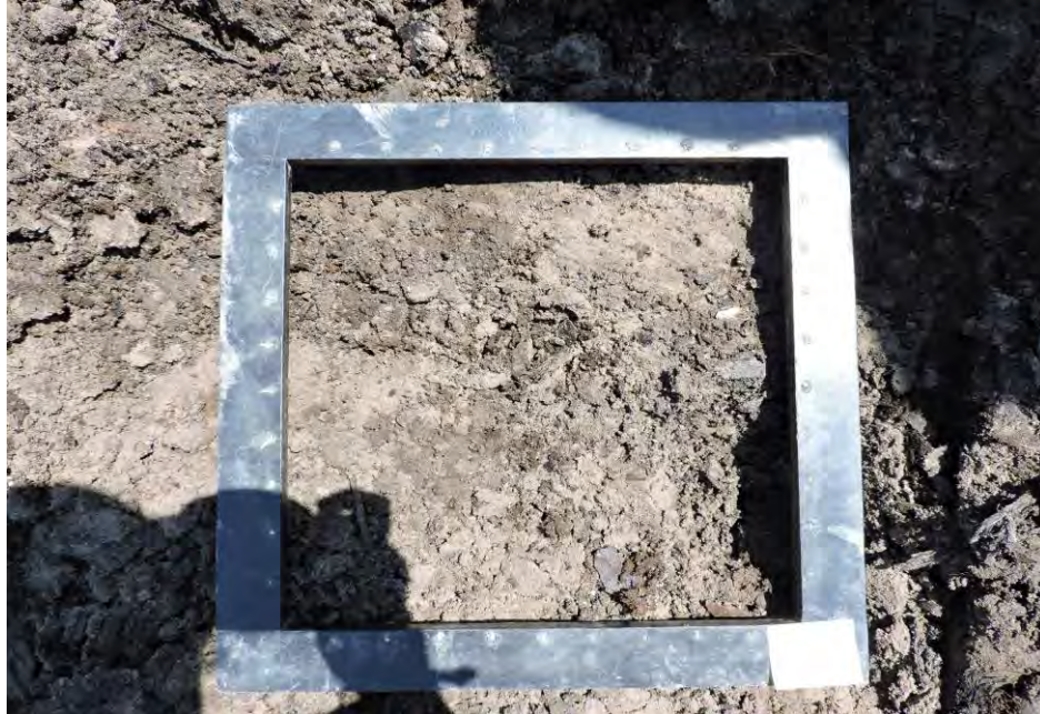
Brown silty fine sand with peat and trace shells
