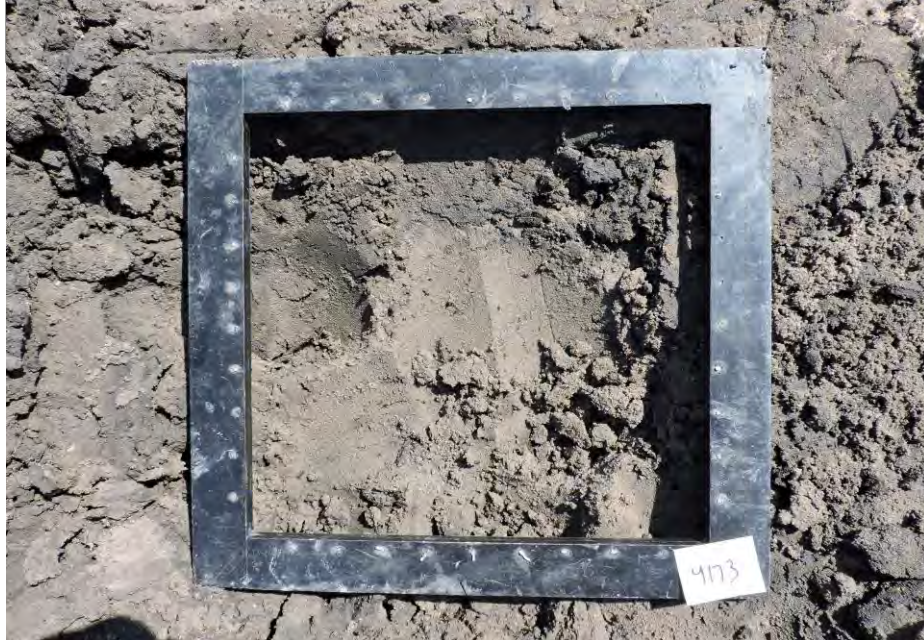
Dark brown silty fine sand with trace shells
