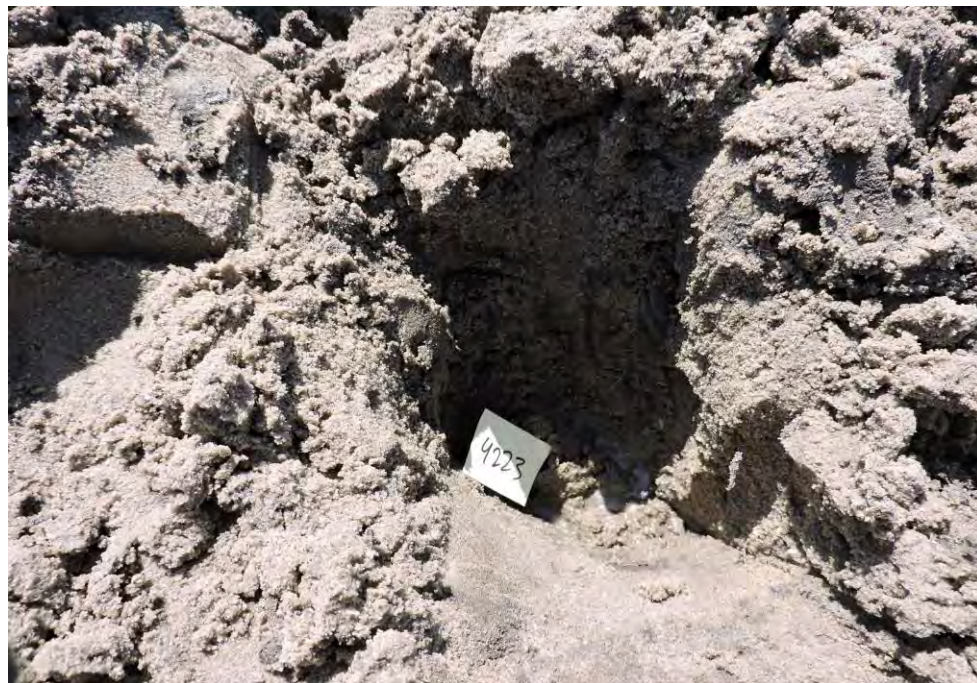
Brown silty fine sand with trace gravel
