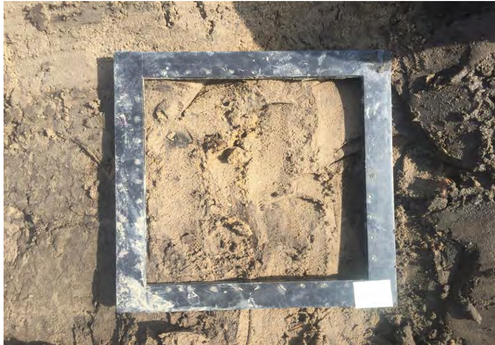
Brown silty fine sand with trace gravel
