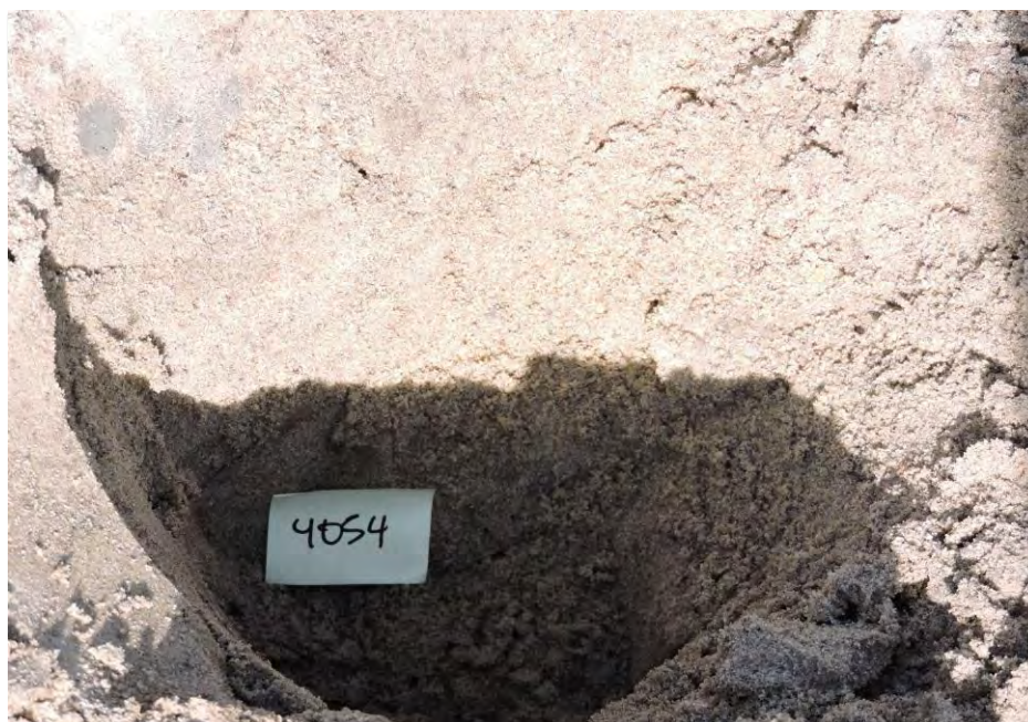
Light-brown silty fine sand with trace shells
