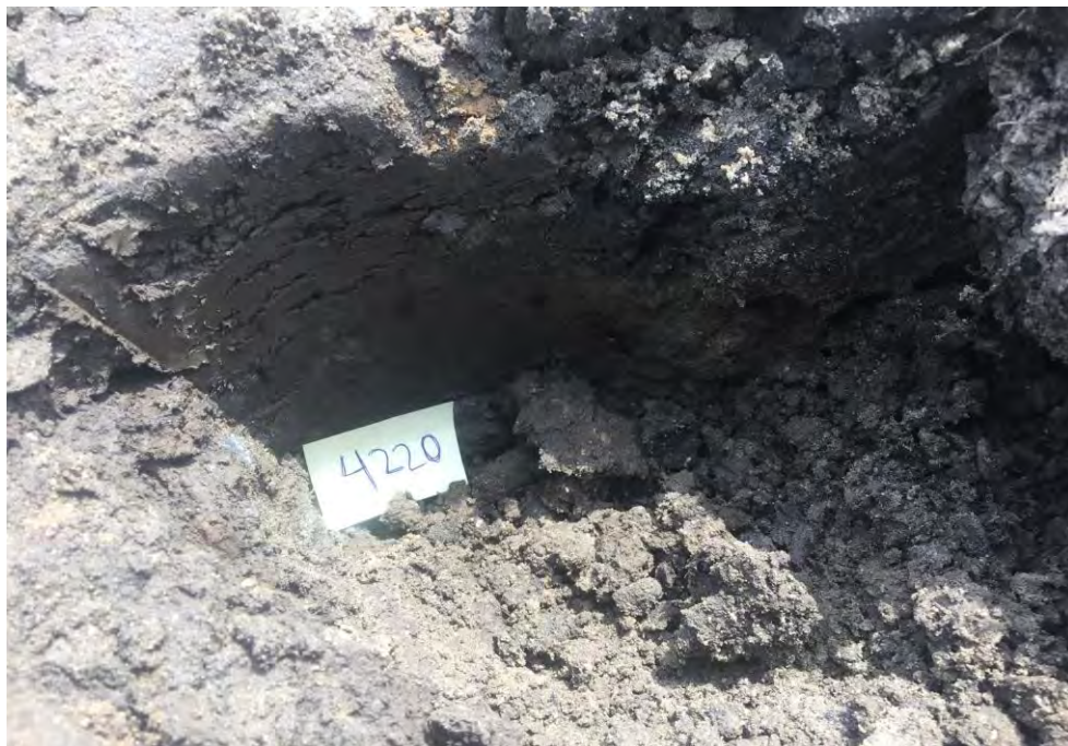
Brown silty fine sand with trace shells
