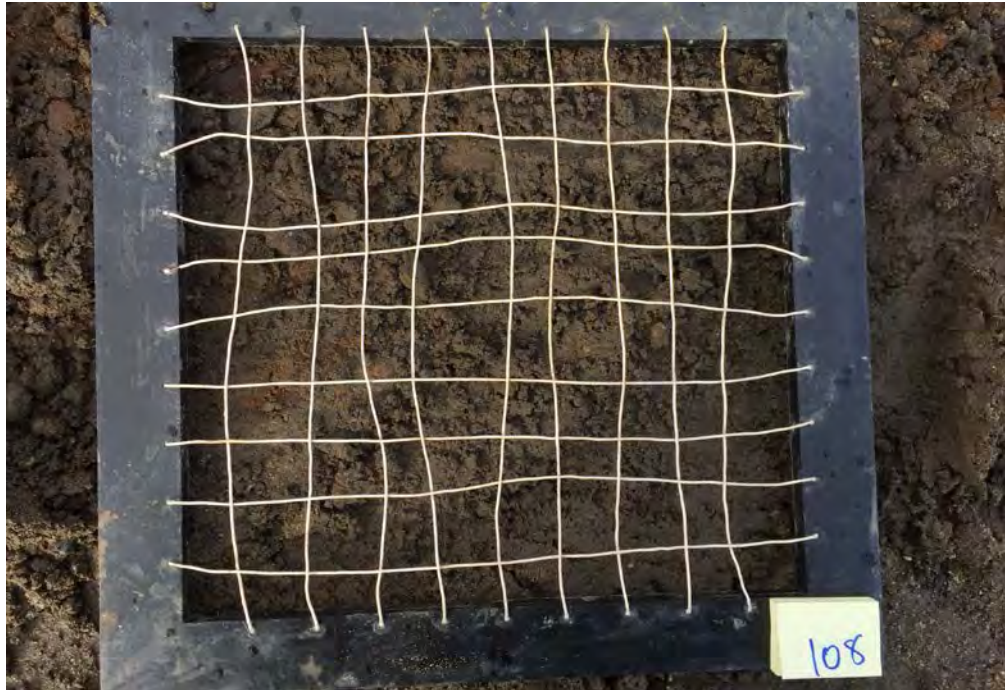
Variegated dark gray-brown silty sand with trace gravel
