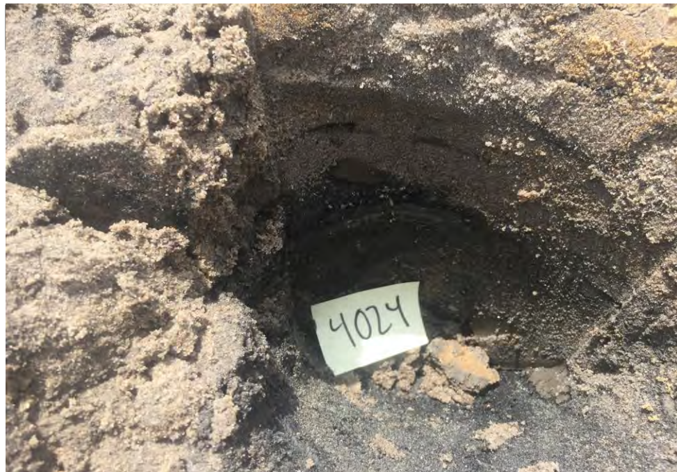
Gray silty fine sand with trace clay and peat
