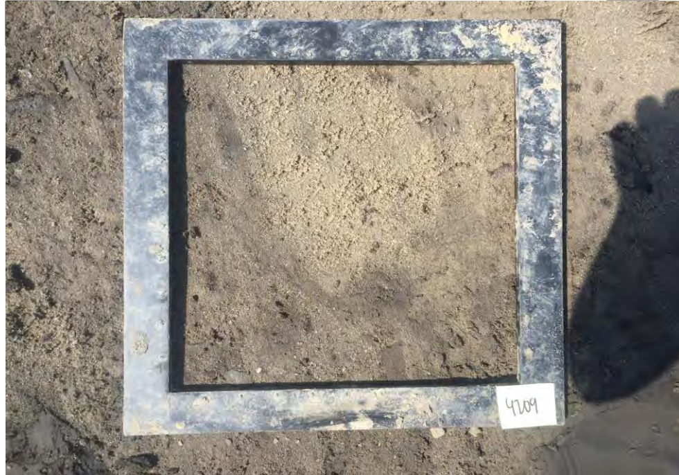
Brown silty fine sand with trace gravel and shells
