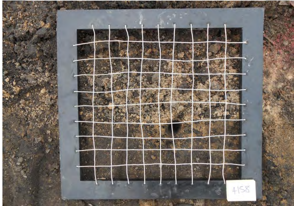
Variegated dark-light brown silty fine sand with trace gravel and sticks
