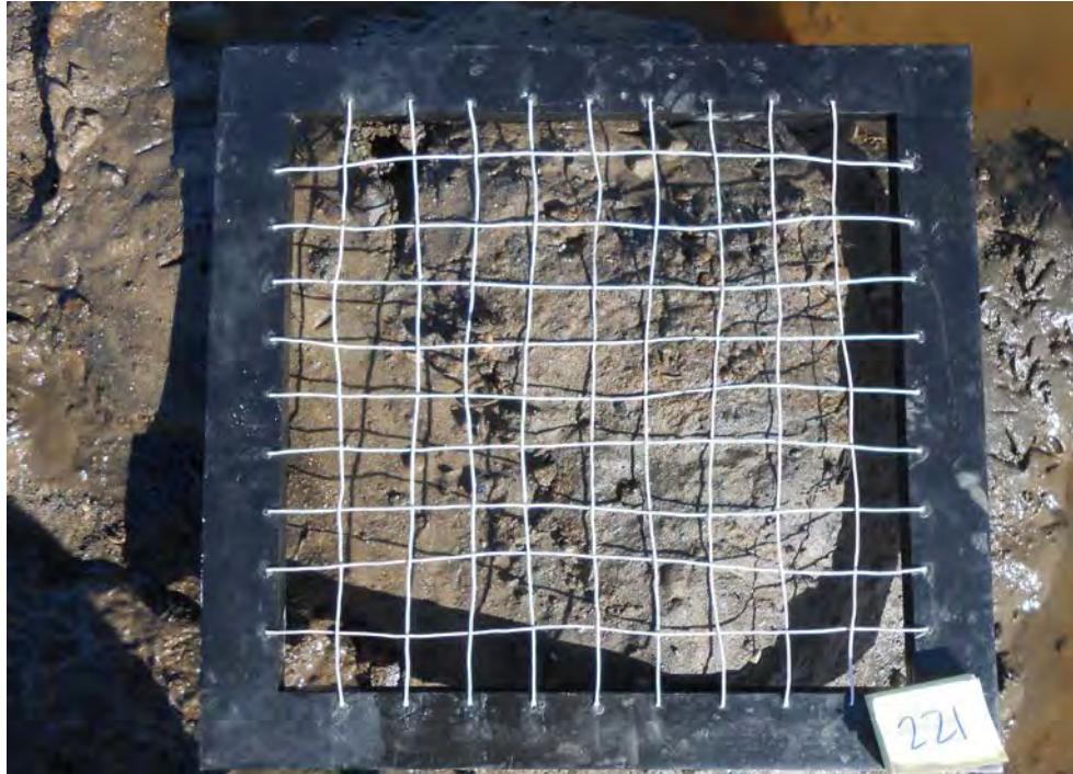
Brown silty fine sand with trace gravel and roots
