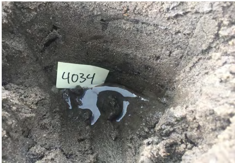
Brown silty fine sand with trace gravel
