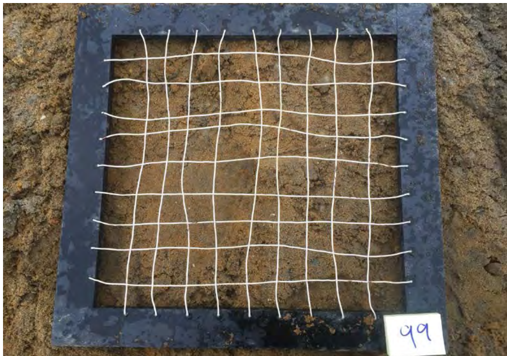
Variegated orange-brown silty fine sand with trace gravel and sticks
