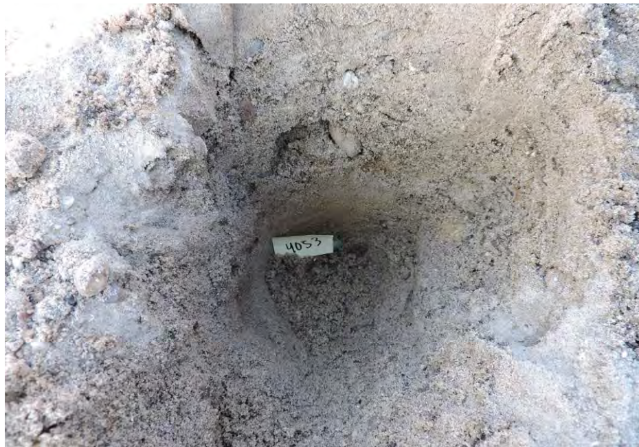
Light brown silty fine sand with little coarse gravel
