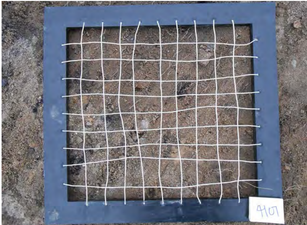
Variegated orange-brown silty fine sand with little coarse gravel and roots and trace clay; some coal chunks (less than 5%). Point 4107 was renumbered to 133 during construction due to the location of the point being outside ash boundaries
