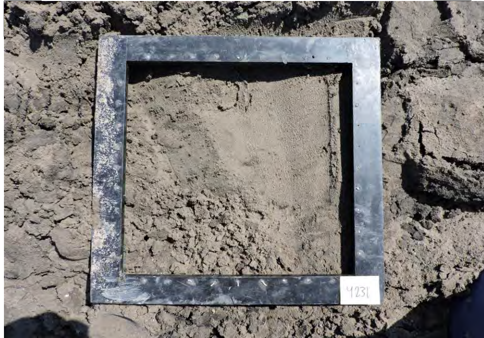
Brown silty fine sand with trace gravel
