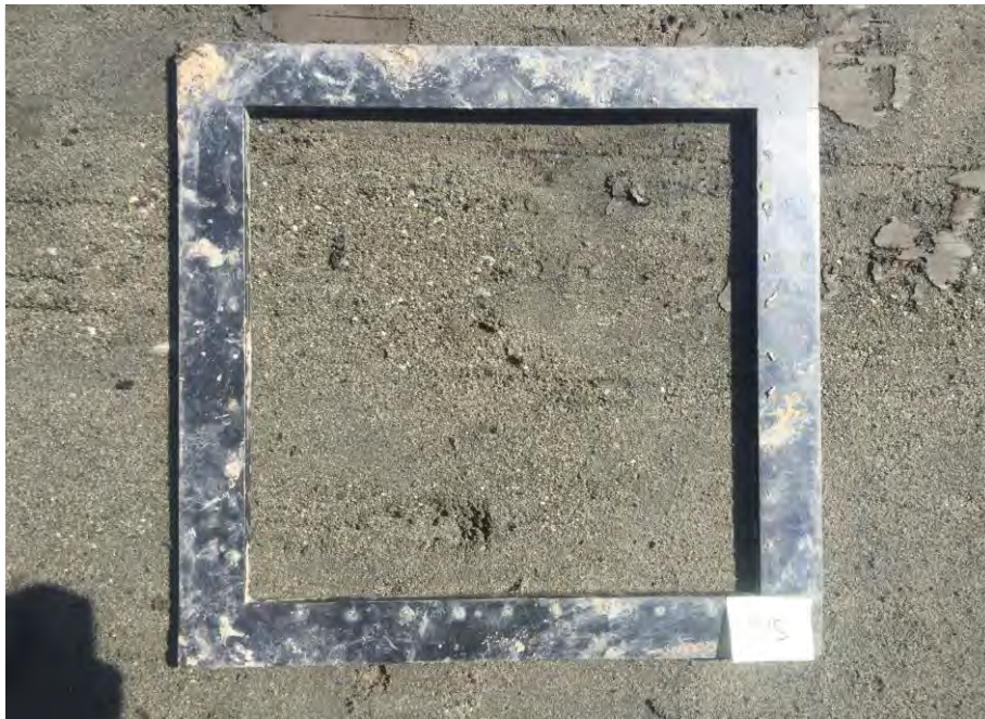
Gray silty fine sand with trace gravel
