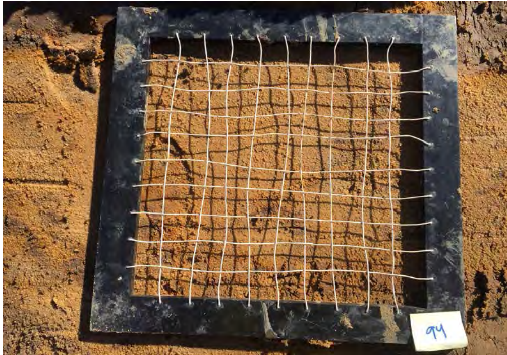
Orange silty fine sand with trace gravel
