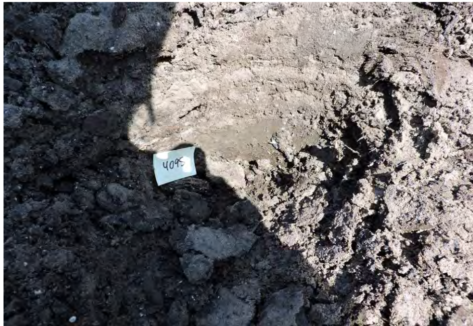
Brown silty fine sand with peat and trace shells
