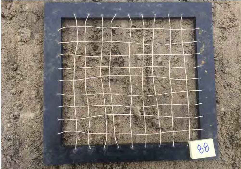
Light gray silty fine sand with trace fine gravel
