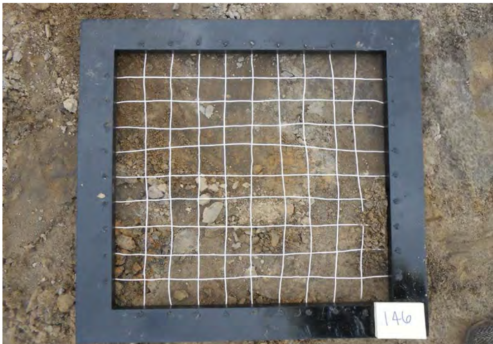
Variegated gray-orange silty fine sand with trace gravel and sticks
