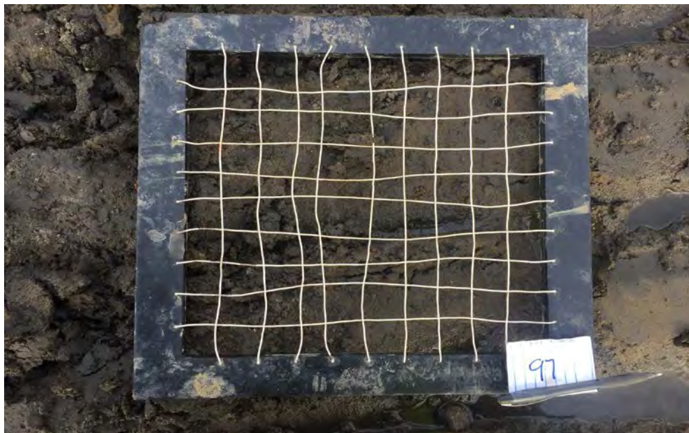
Variegated gray-brown silty fine sand with trace gravel
