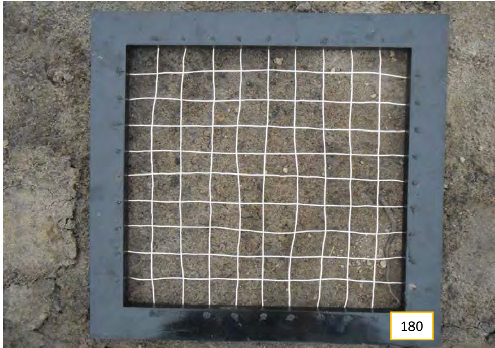
Gray silty fine sand with trace gravel and roots
