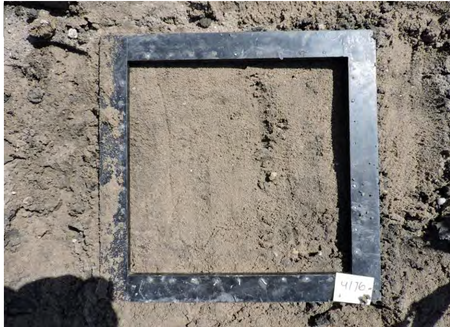
Medium-dark brown silty fine sand with trace shells and sticks
