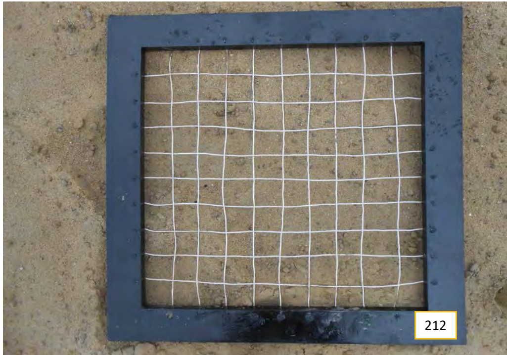
Light brown silty fine sand with trace fine gravel
