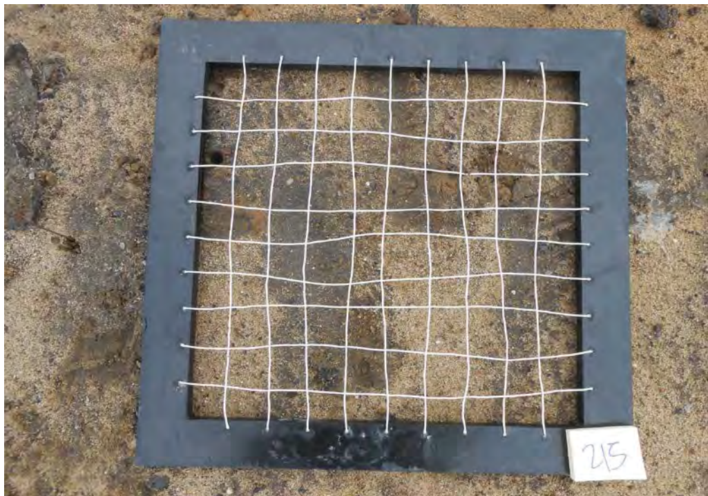
Brown silty fine sand with trace gravel and sticks
