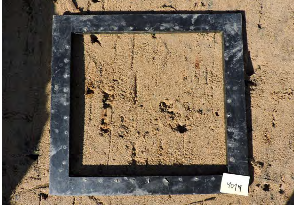
Medium brown silty fine sand with trace gravel
