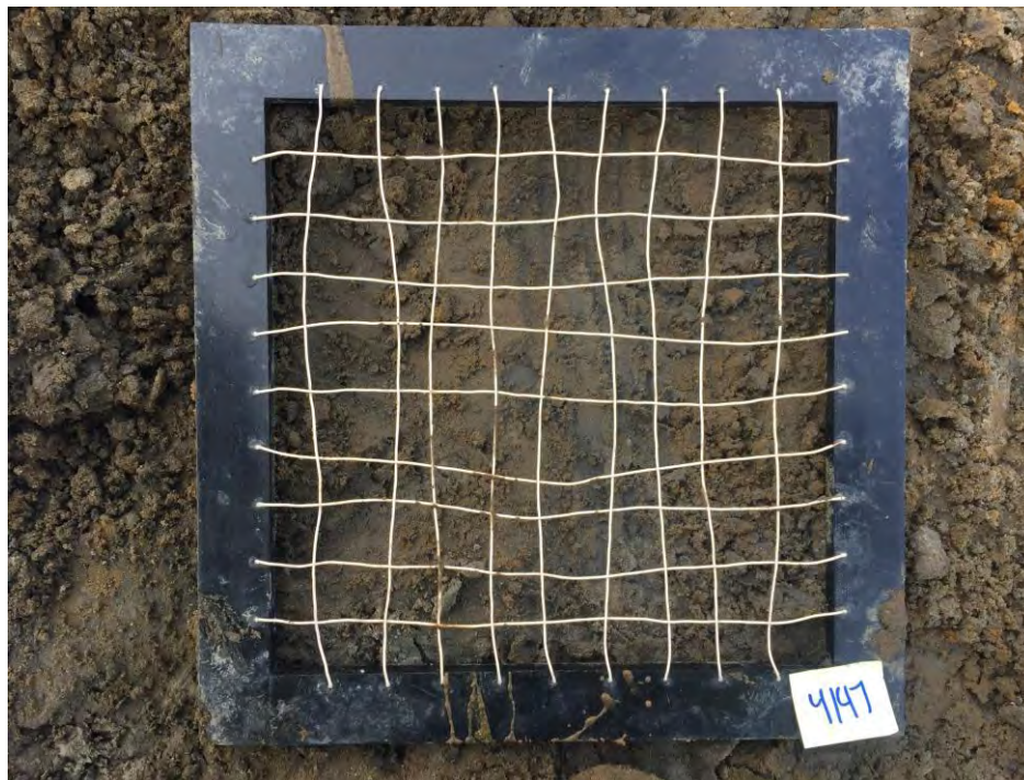
Variegated brown-light gray silty fine sand with trace gravel
