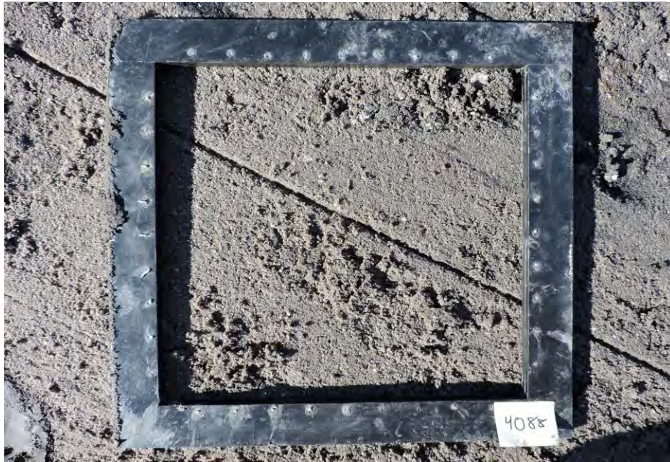
Brown silty fine sand with some clay and trace peat
