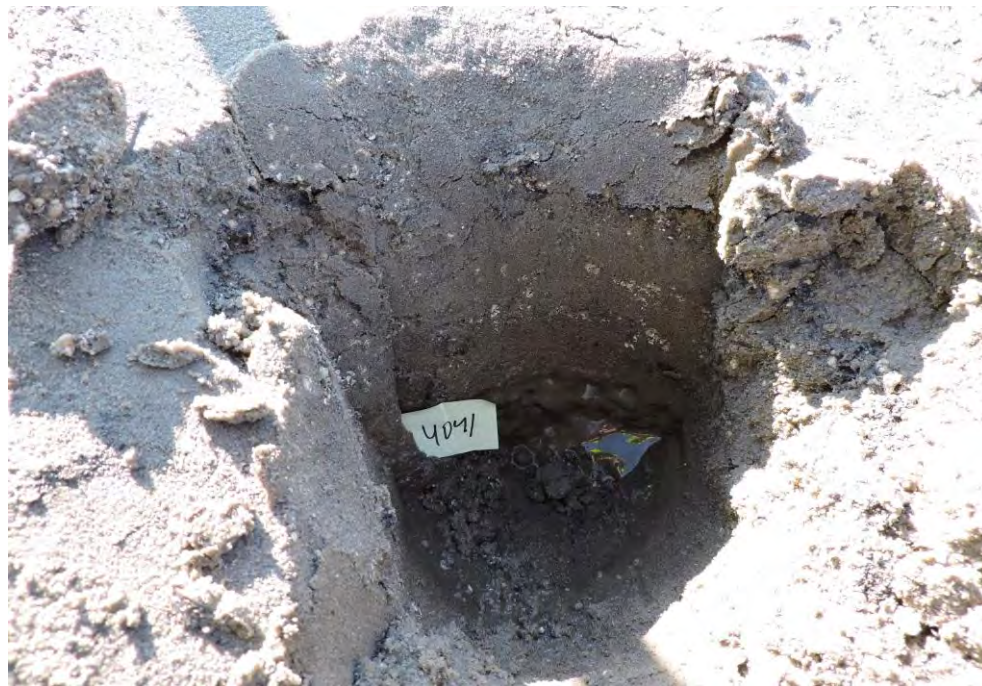
Medium brown silty fine sand with some shells
