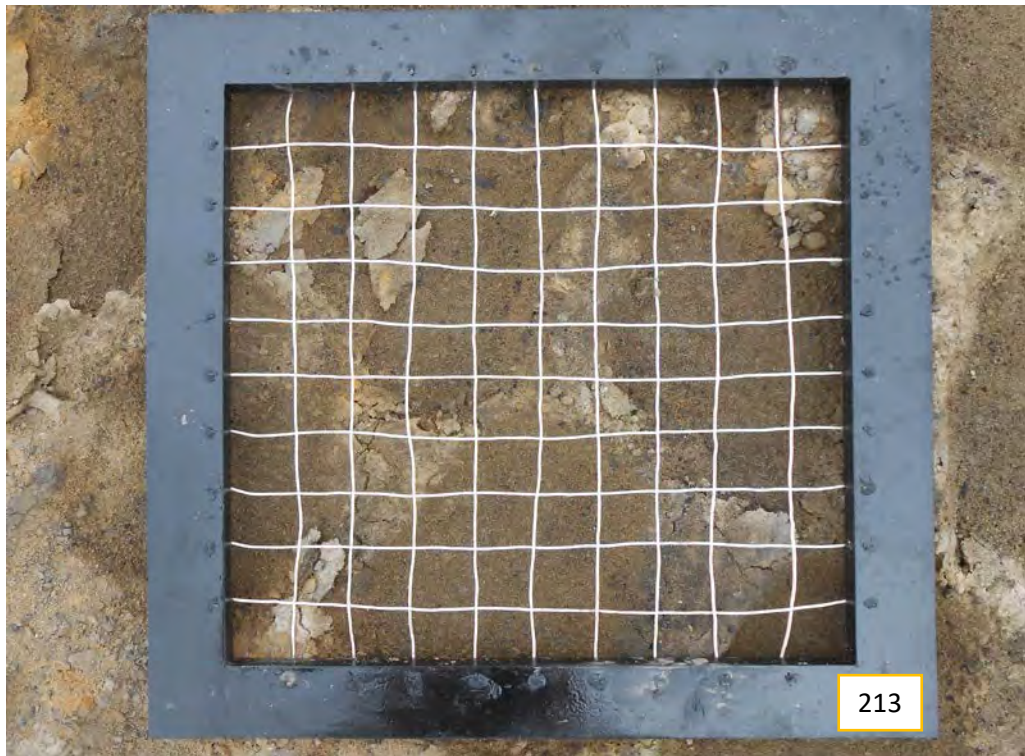
Variegated light brown-orange silty fine sand with trace gravel
