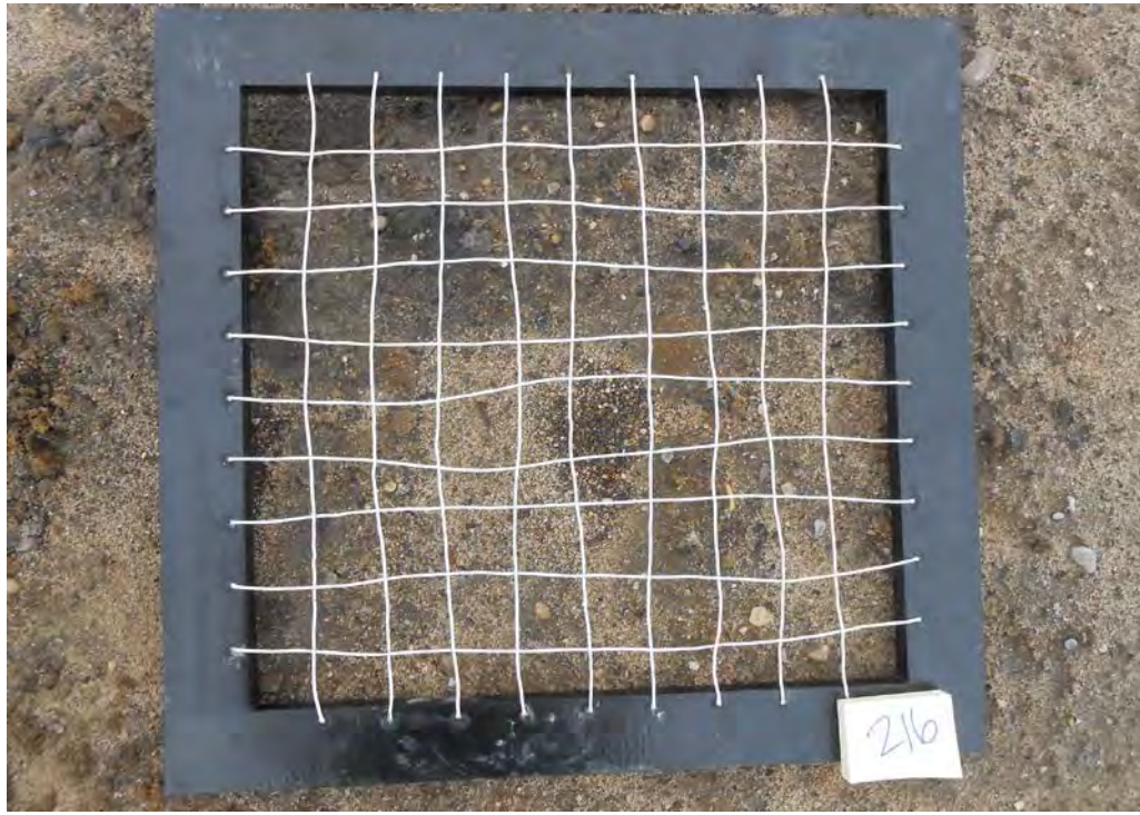
Variegated light brown-dark gray silty fine sand with trace gravel
