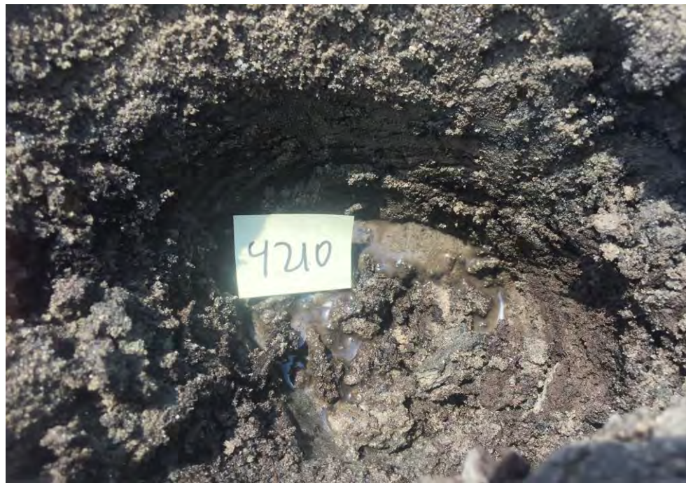
Brown silty fine sand with trace gravel
