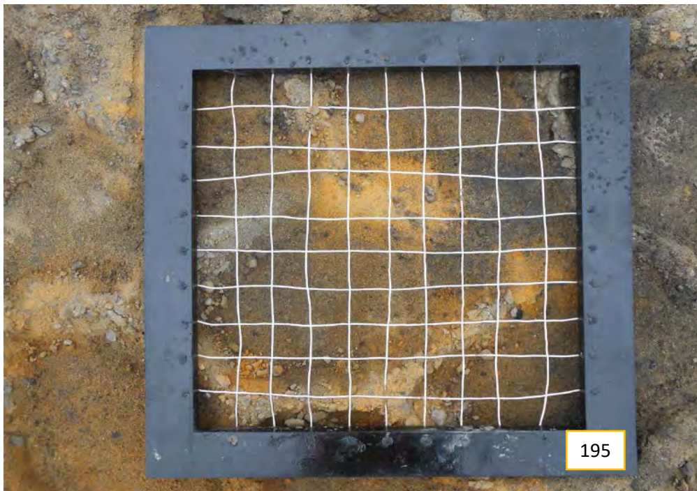
Variegated orange-brown-gray silty fine sand with grace gravel
