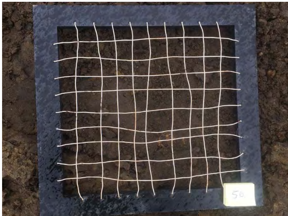
Dark brown silty fine sand with trace gravel
