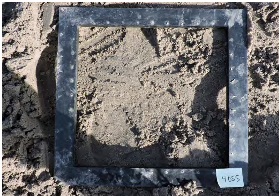
Medium brown silty fine sand with trace shells
