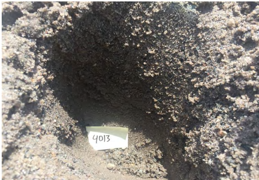
Brown silty fine ssand with some gravel
