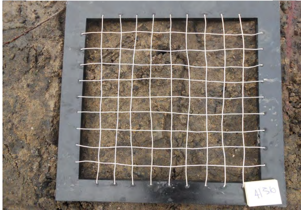
Variegated light-dark brown silty fine sand with trace gravel
