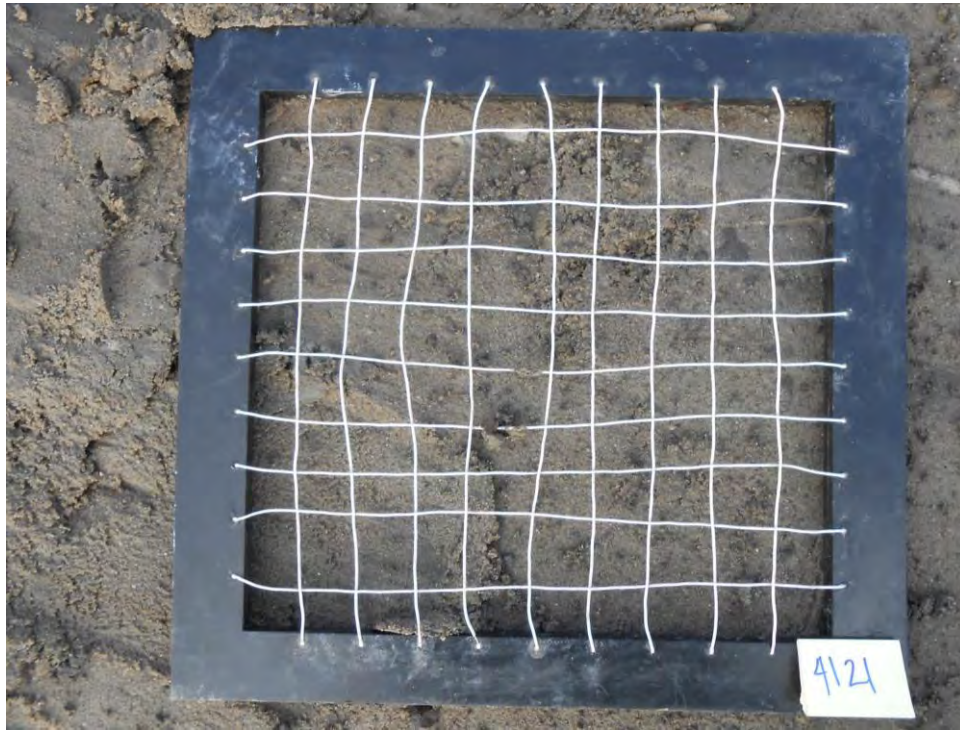
Gray silty fine sand with trace gravel
