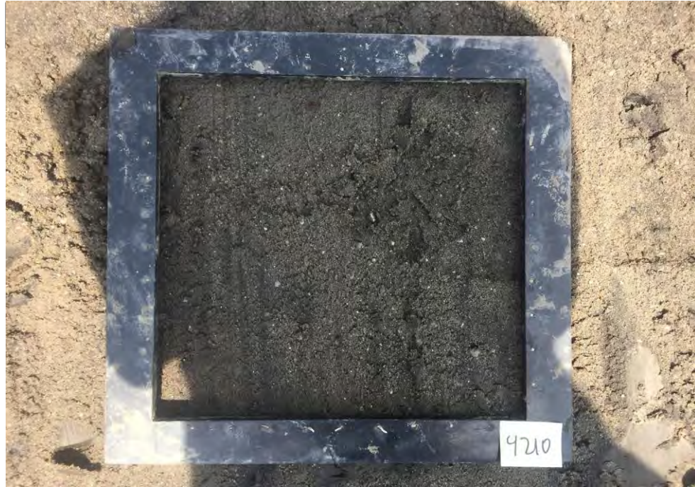
Brown silty fine sand with trace gravel
