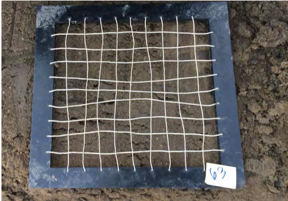
Gray silty fine sand with trace gravel
