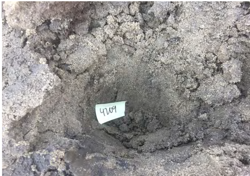
Brown silty fine sand with trace gravel and shells
