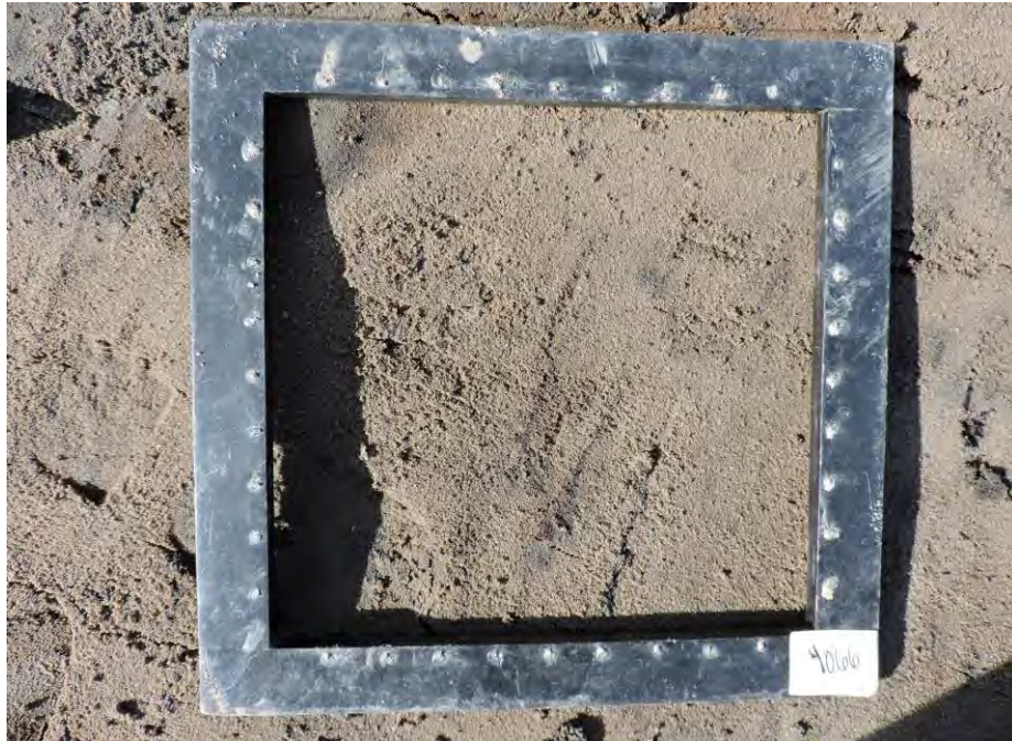
Brown silty fine sand with trace clay
