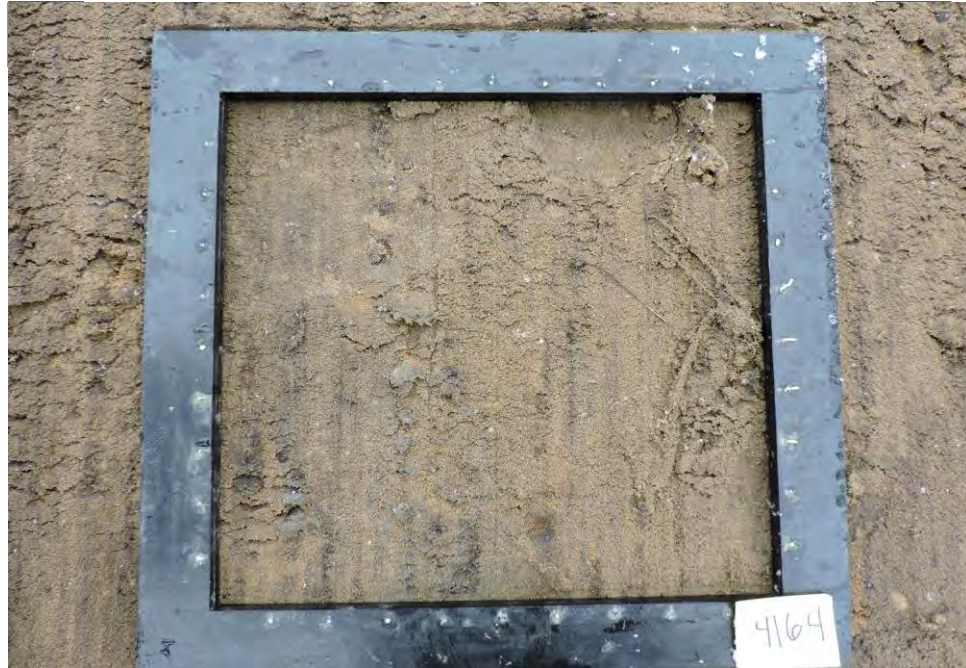
Brown silty fine sand with trace clay
