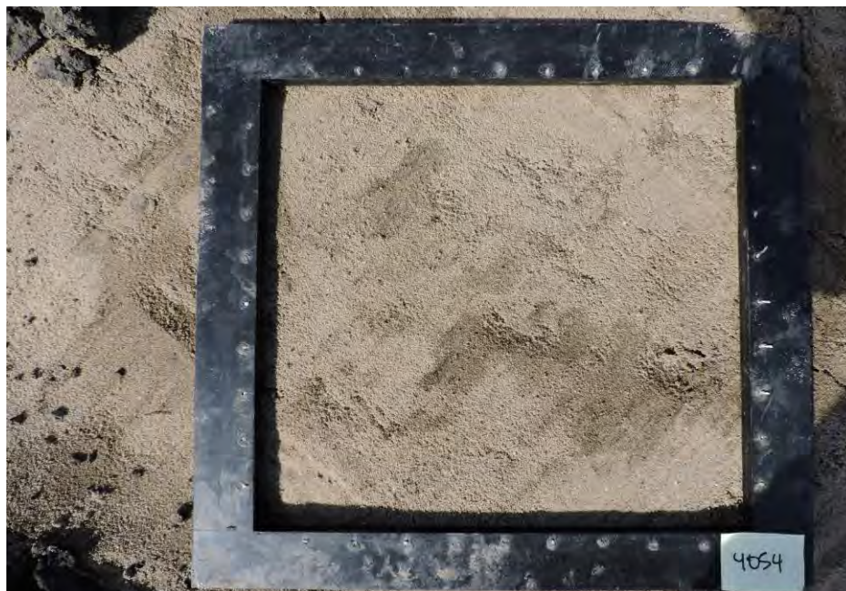
Light-brown silty fine sand with trace shells
