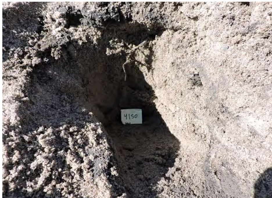
Light brown silty fine sand with trace gravel
