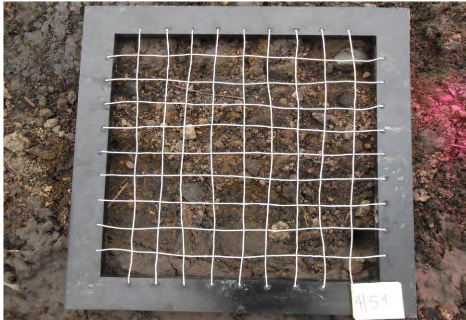
Variegated orange-dark gray silty fine sand with trace gravel and roots
