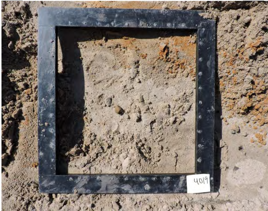
Brown-orange silty fine sand with trace gravel
