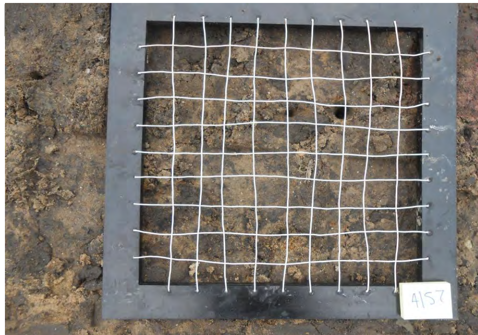
Variegated gray-brown silty fine sand with trace gravel and sticks
