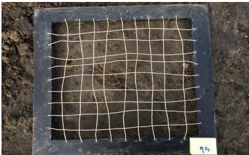
Gray silty fine sand with trace clay
