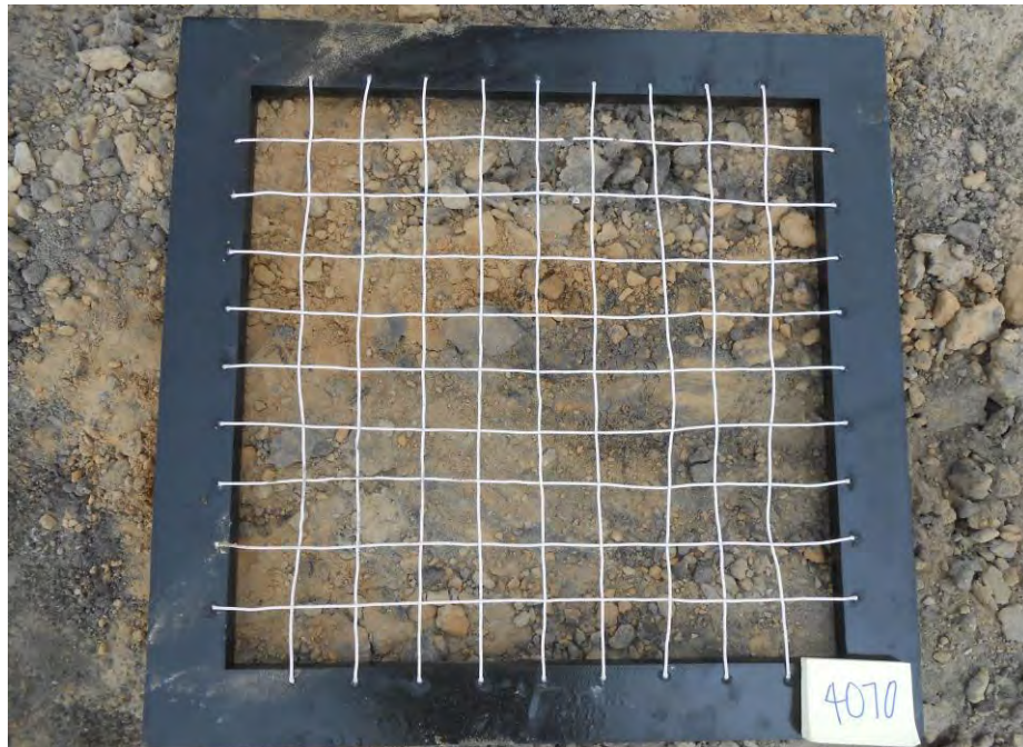
Variegated gray-brown silty fine sand with trace coarse gravel and sticks
