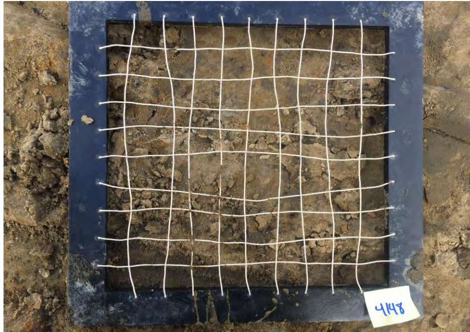
Variegated light brown-light gray silty fine sand with trace gravel
