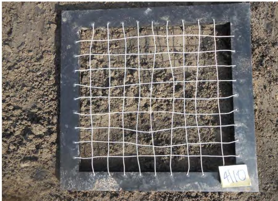
Gray silty fine sand with trace gravel
