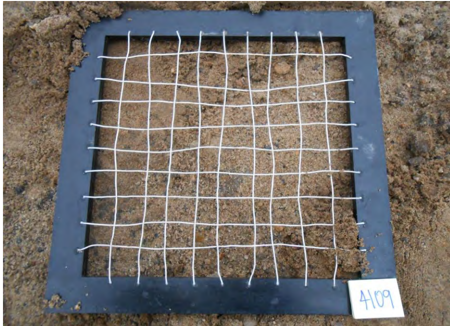
Brown silty fine sand with trace gravel
