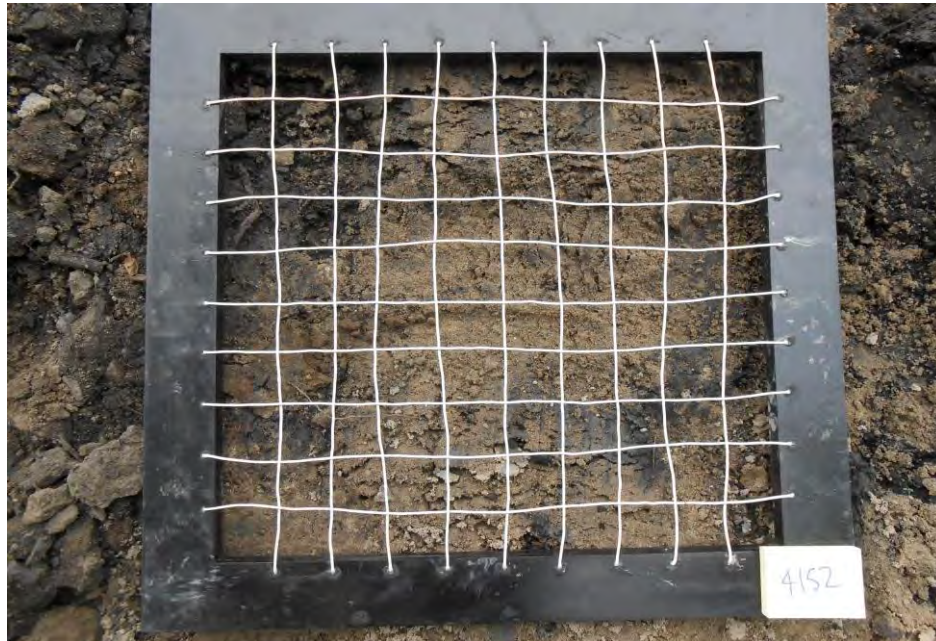
Brown silty fine sand with trace gravel
