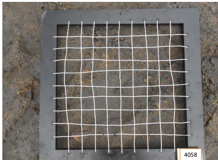
Variegated gray-brown silty fine sand with trace gravel and sticks
