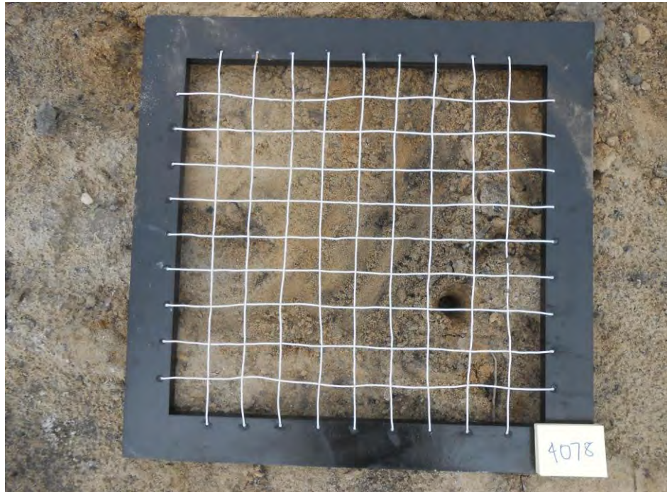
Variegated light gray-brown silty fine sand with trace gravel and roots
