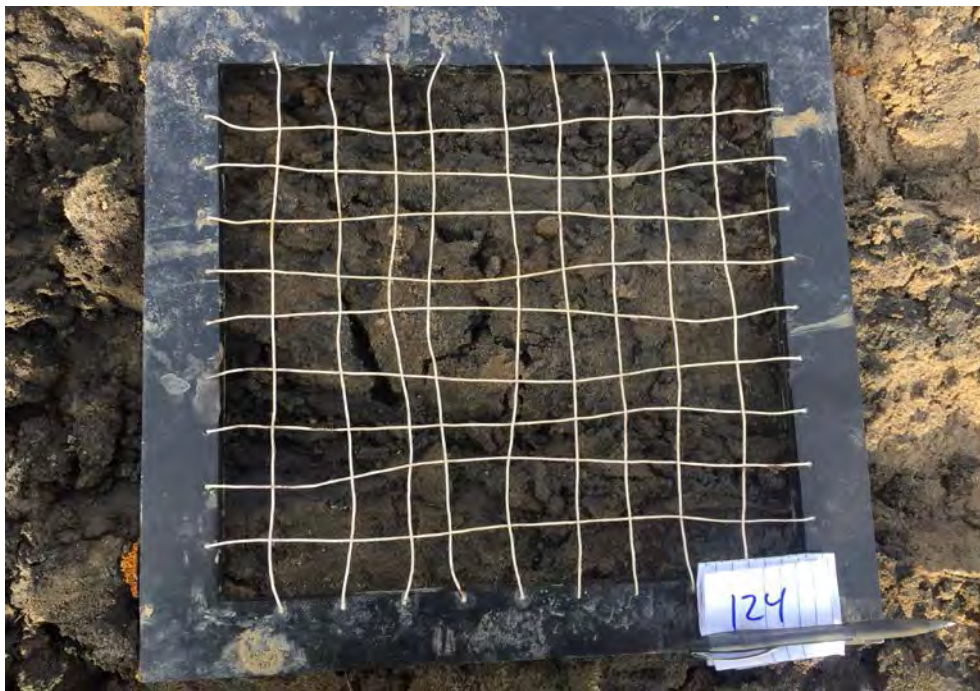
Brown silty fine sand with trace gravel sticks and roots
