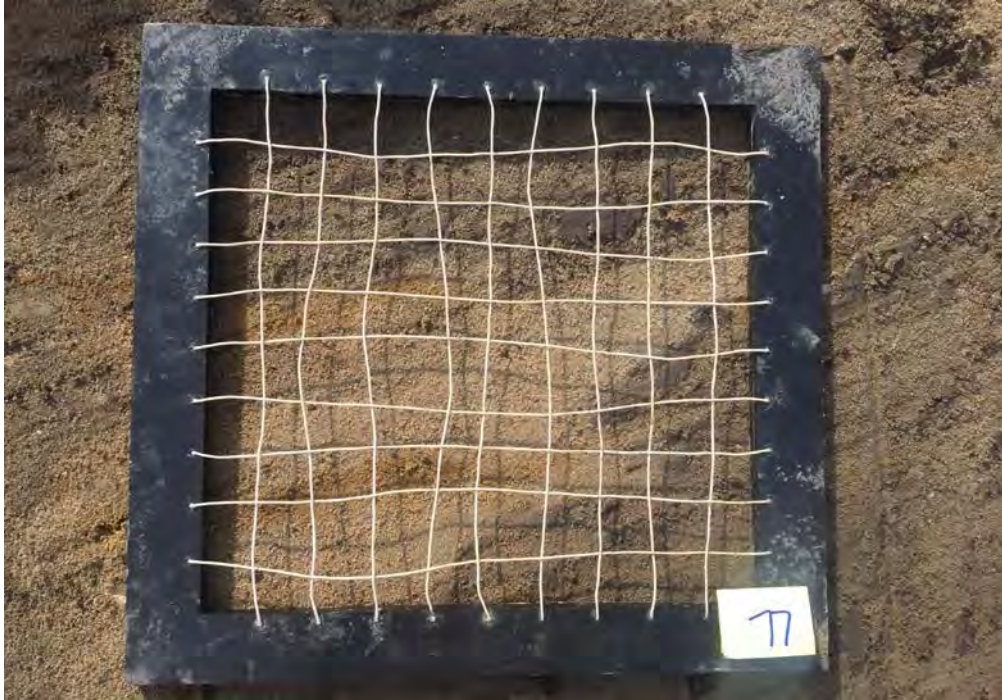
Variegated orange-brown silty fine sand with trace clay
