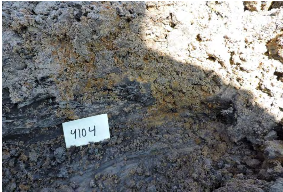
Brown-orange silty fine sand with peat layers
