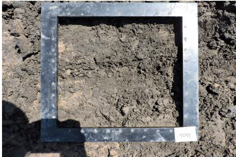
Brown silty fine sand with trace gravel
