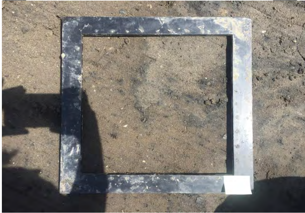
Brown silty fine sand with trace gravel and sand
