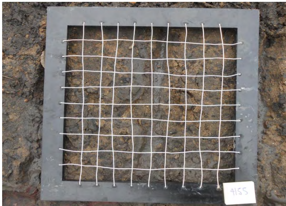
Variegated light-dark brown silty fine sand with trace gravel and roots
