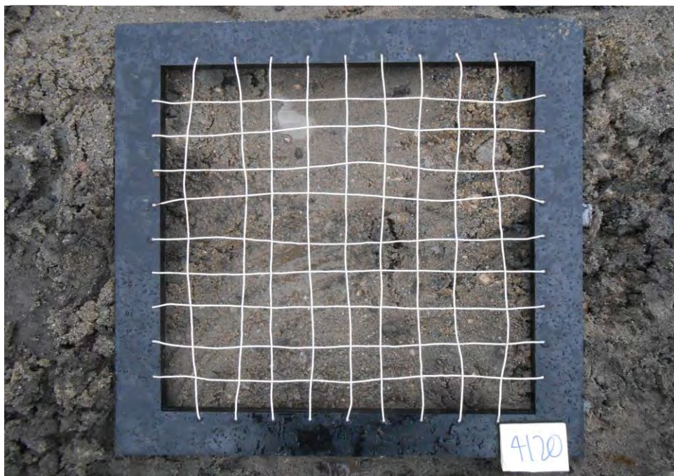
Variegated gray-brown silty fine sand with trace gravel
