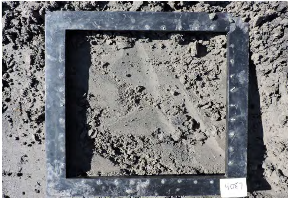
Gray silty fine sand with trace gravel and some peat
