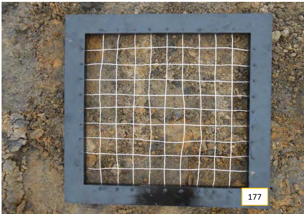
Variegated brown-gray silty fine sand with trace gravel
