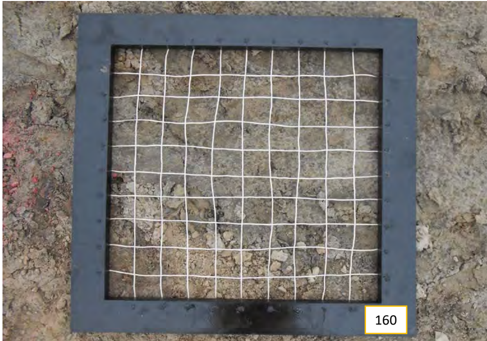
Variegated light gray-light brown silty fine sand with trace gravel
