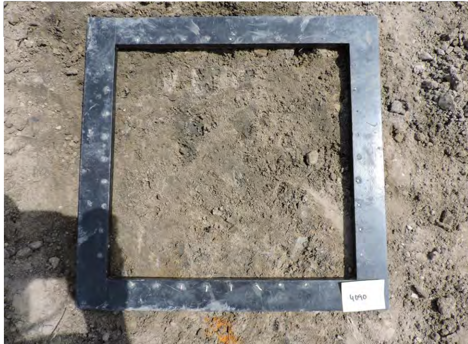
Medium brown silty fine sand with trace gravel
