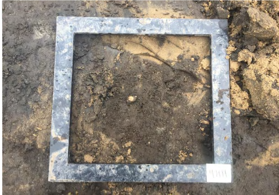
Light-dark brown silty fine sand with trace shells
