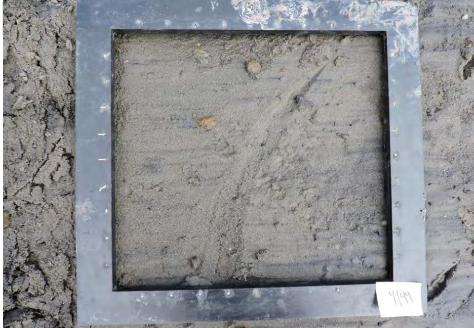
Dark gray silty fine sand with trace peat and trace clay
