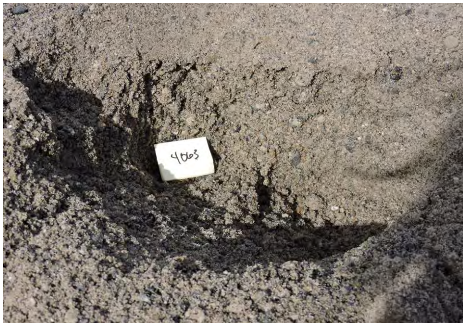
Light brown silty fine sand with some gravel
