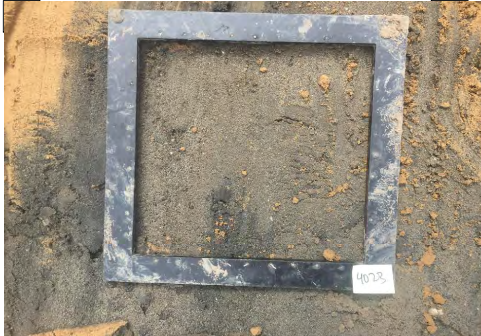
Gray silty fine sand with trace gravel
