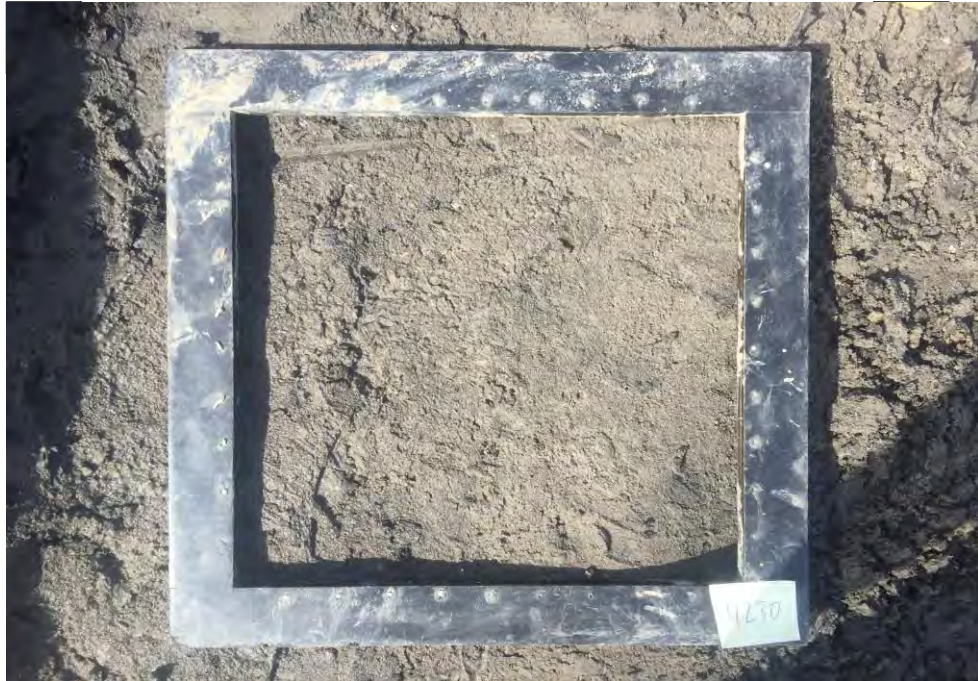
Gray silty fine sand with trace gravel and shells
