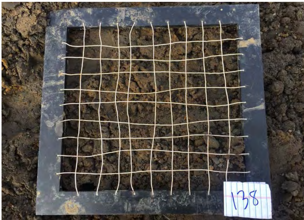
Brown silty fine sand with trace gravel
