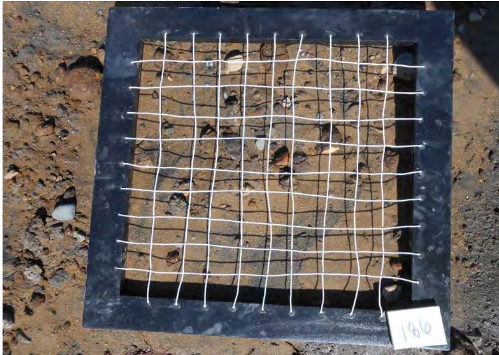
Variegated gray-brown silty fine sand with trace coarse gravel
