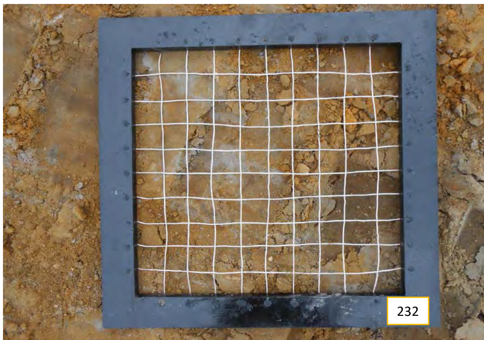
Variegated orange-gray silty fine sand with trace gravel
