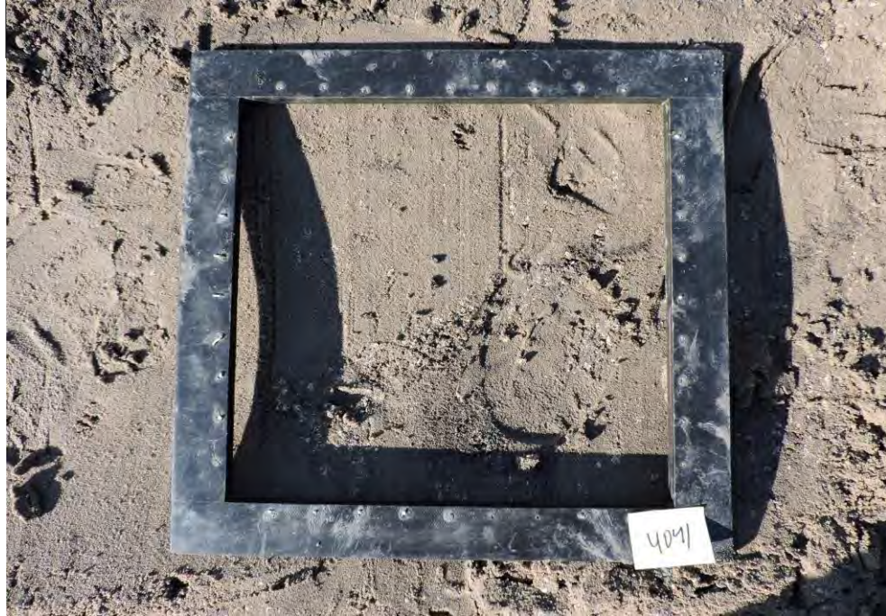
Medium brown silty fine sand with some shells
