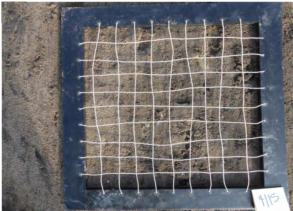
Gray silty fine sand with trace clay
