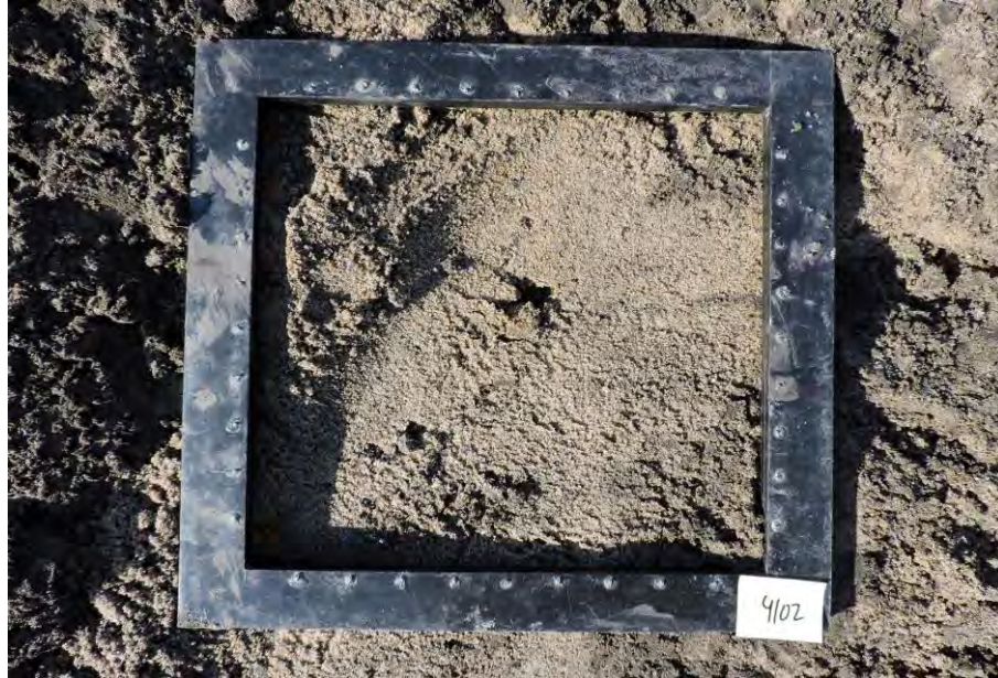
Medium brown silty fine sand with trace gravel
