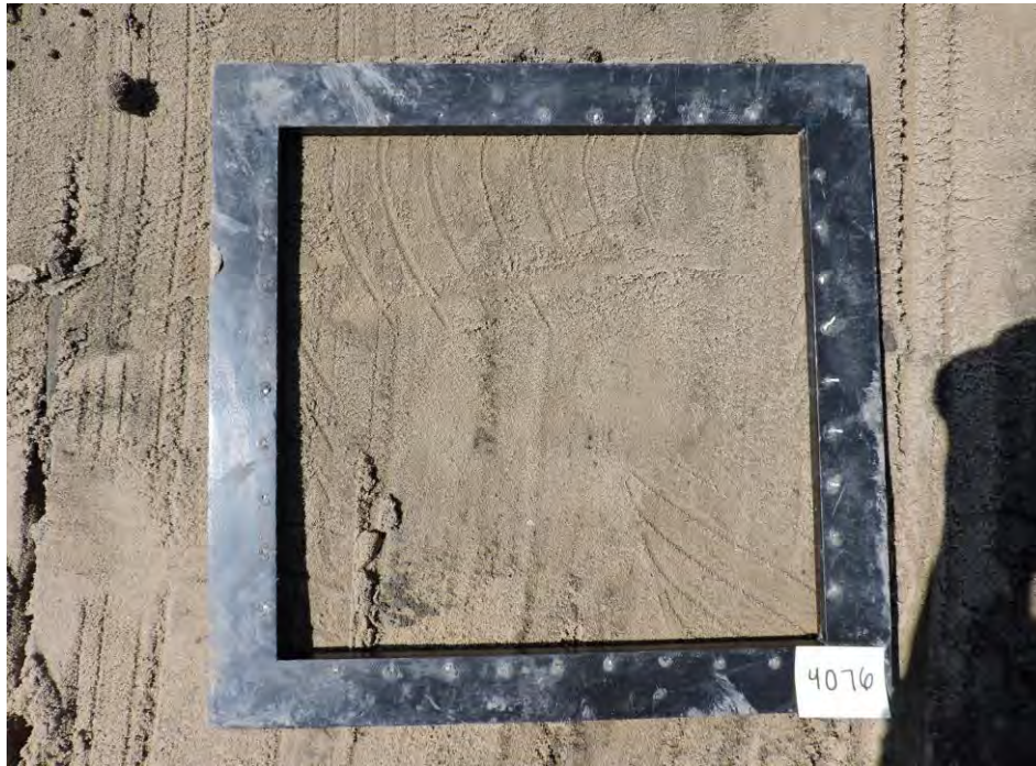
Light-dark brown silty fine sand with trace gravel
