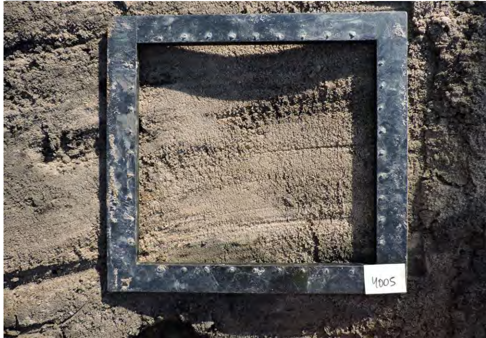
Brown silty fine sand with trace clay
