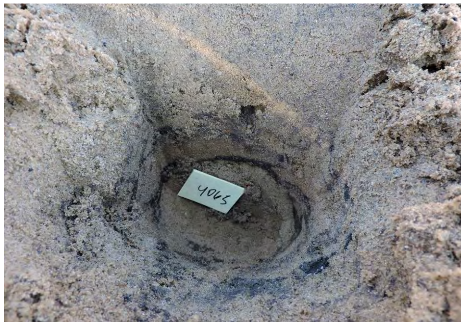
Light brown silty fine sand with trace gravel
