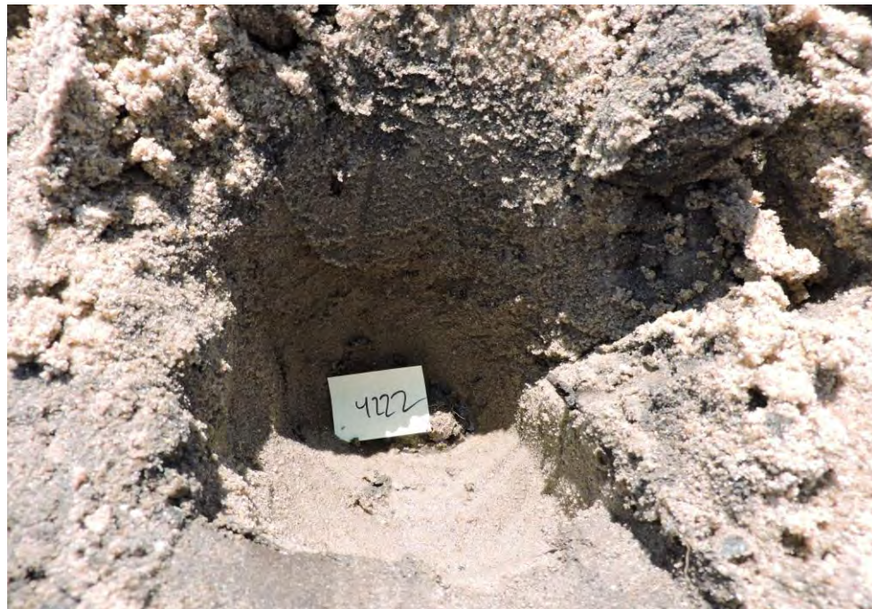
Brown silty fine sand with trace gravel
