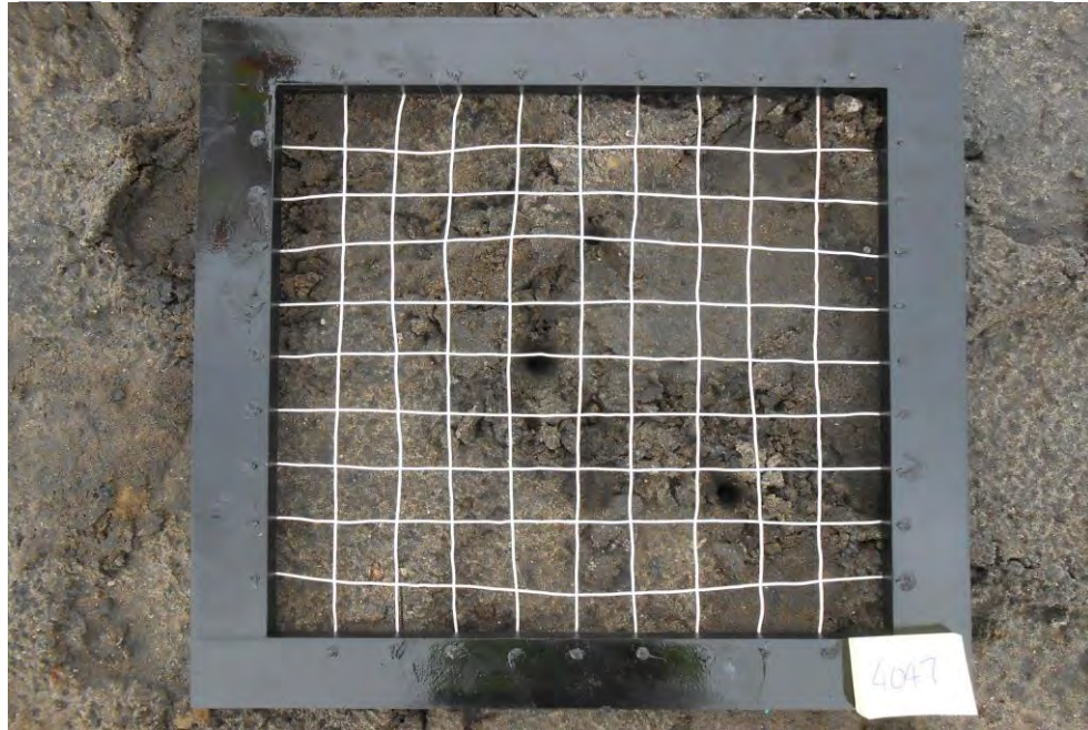
Variegated gray-brown silty fine sand with trace gravel and sticks
