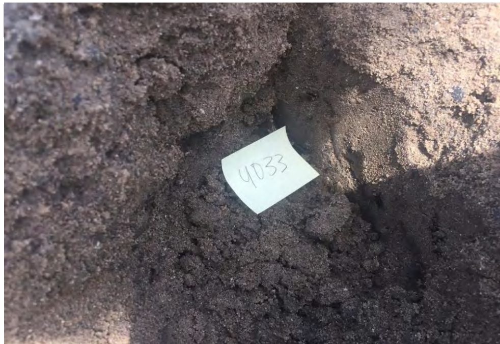
Brown silty fine sand with trace gravel
