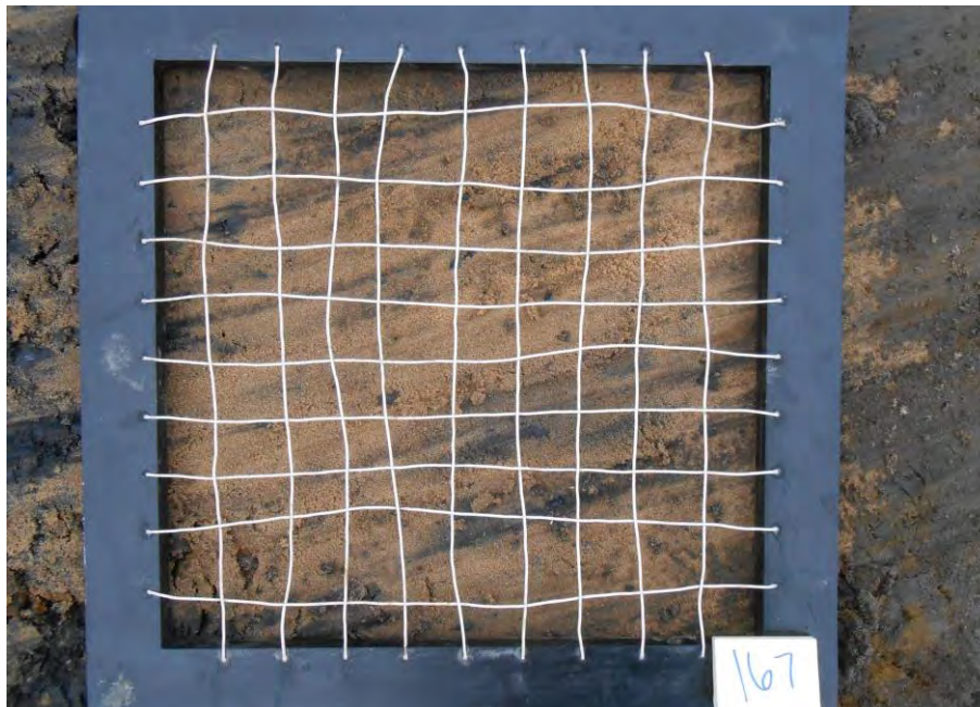
Variegated light brown-dark gray silty fine sand. Point 167 was renumbered to 4113 during construction due to the location of the point being within ash boundaries.
