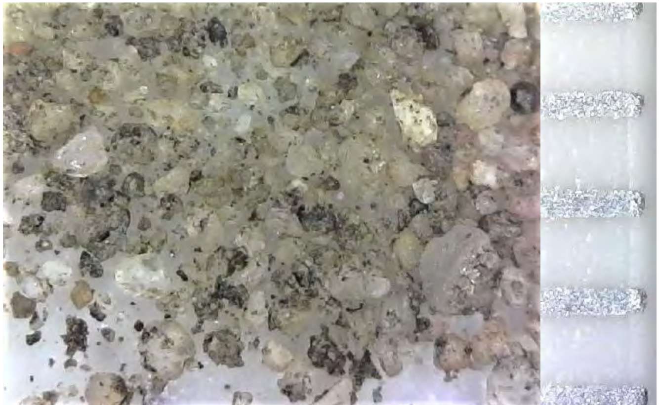
Soil from Sample Location 5076A-1 (1.2 – 1.6') [Scale marks are each 1 mm]
