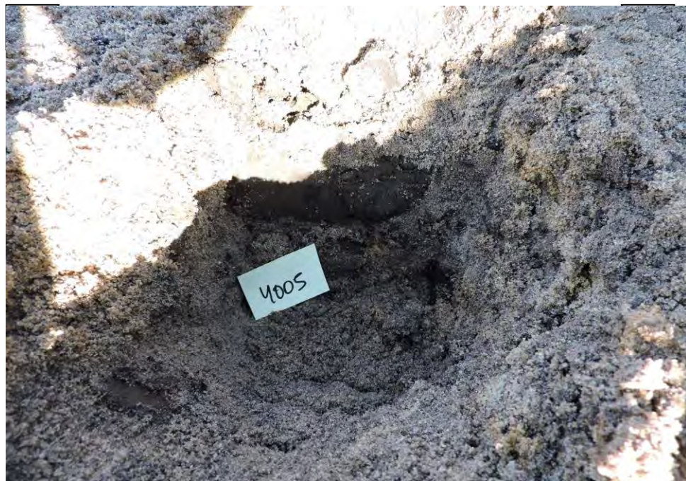
Brown silty fine sand with trace clay
