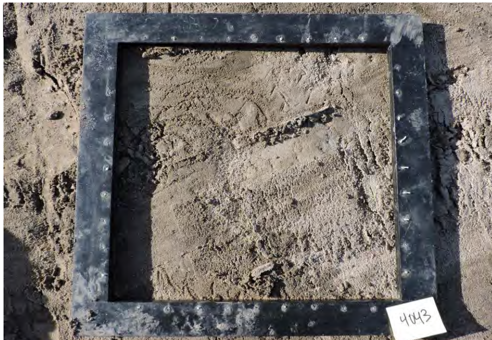
Light-dark brown silty fine sand with trace clay and roots
