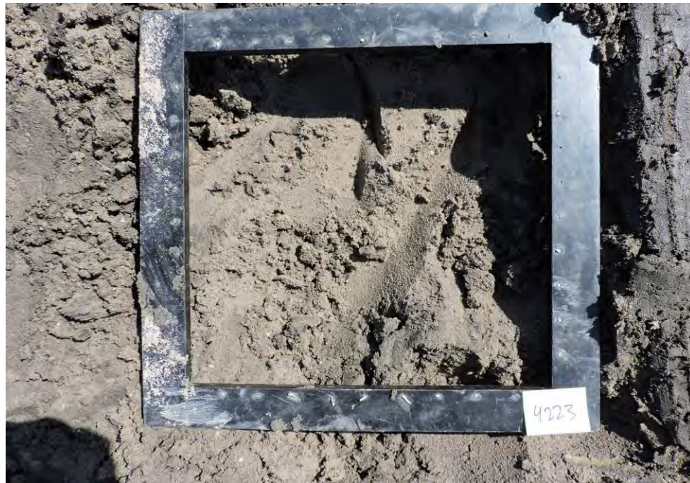
Brown silty fine sand with trace gravel
