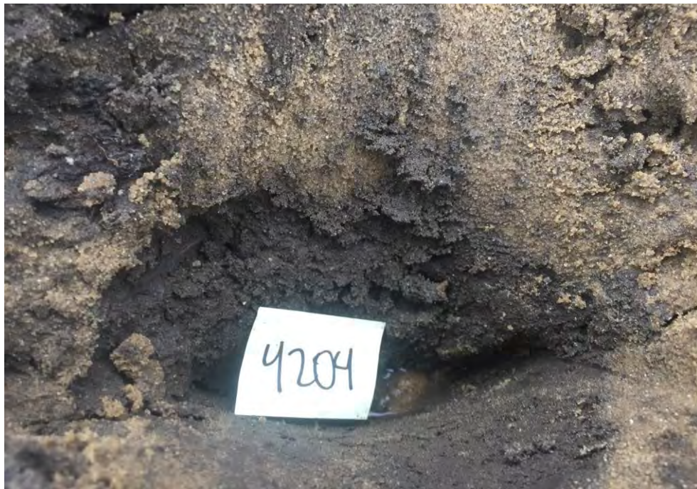
Light-dark brown silty fine sand with trace shells
