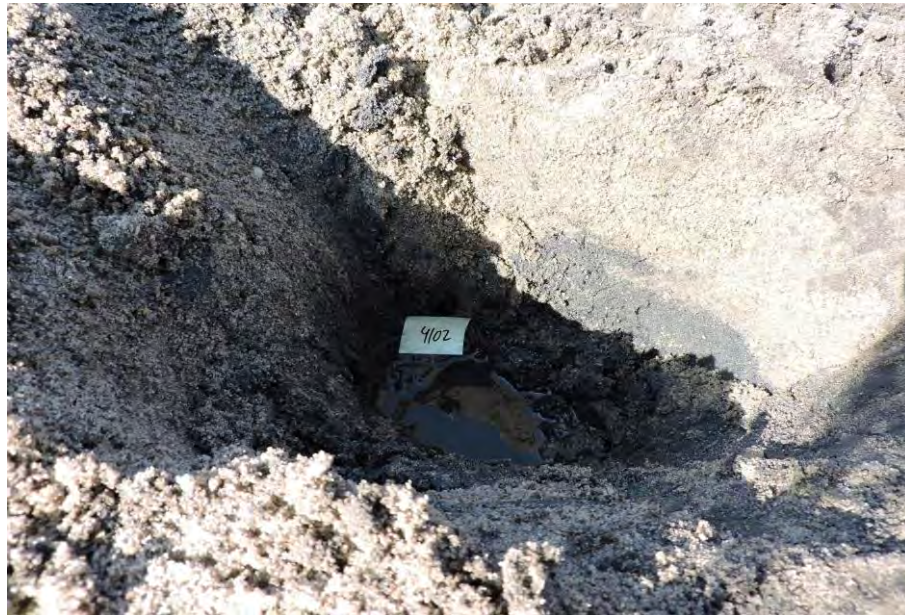
Medium brown silty fine sand with trace gravel
