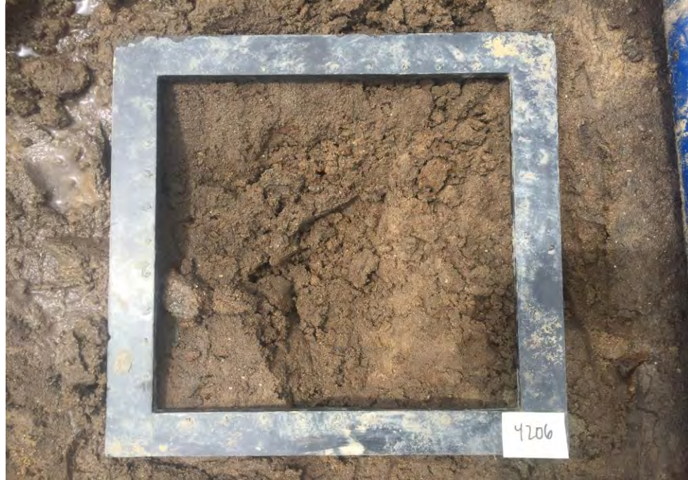
Brown silty fine sand with trace gravel
