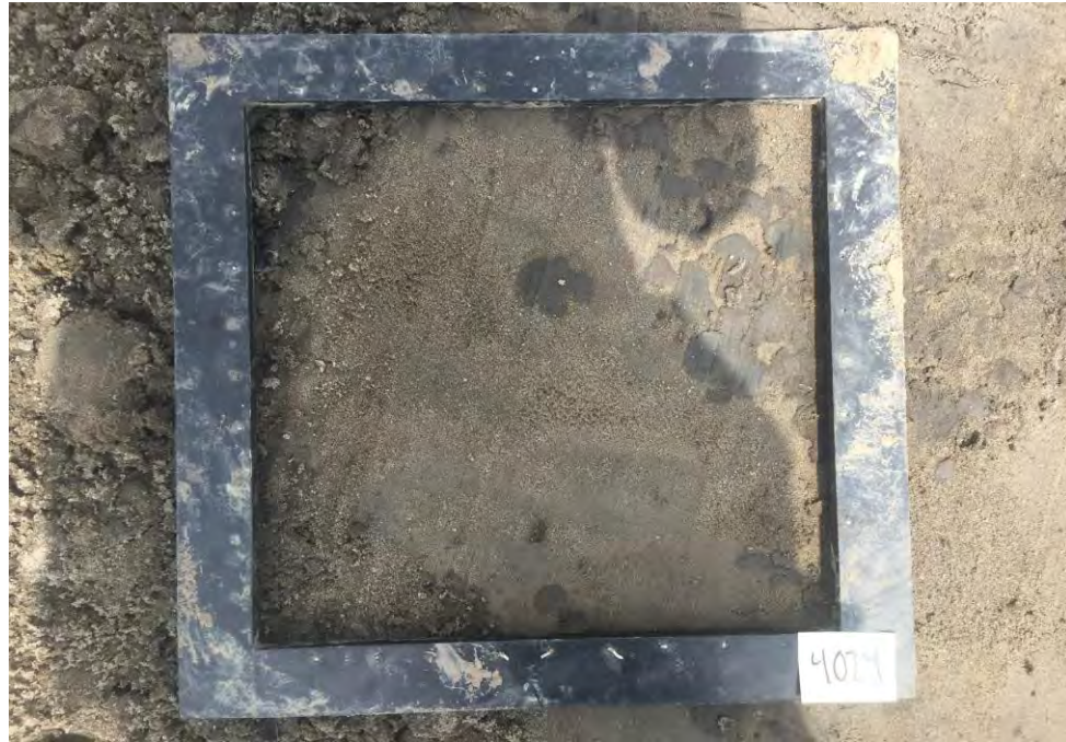
Gray silty fine sand with trace clay and peat
