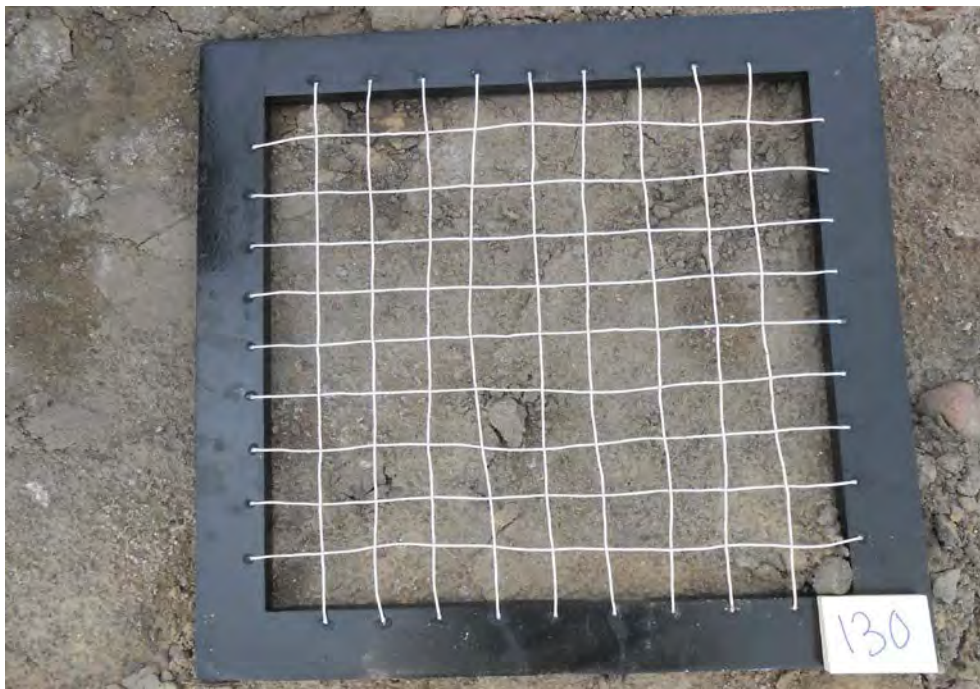
Light gray silty fine sand with little coarse gravel
