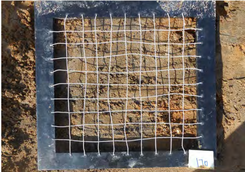
Brown silty fine sand with trace clay
