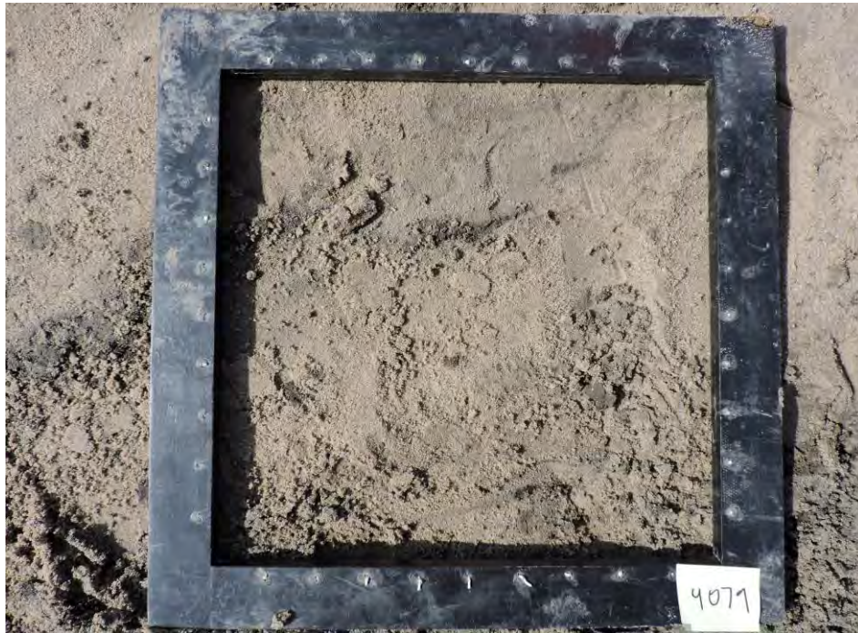
Light brown silty fine sand with trace clay
