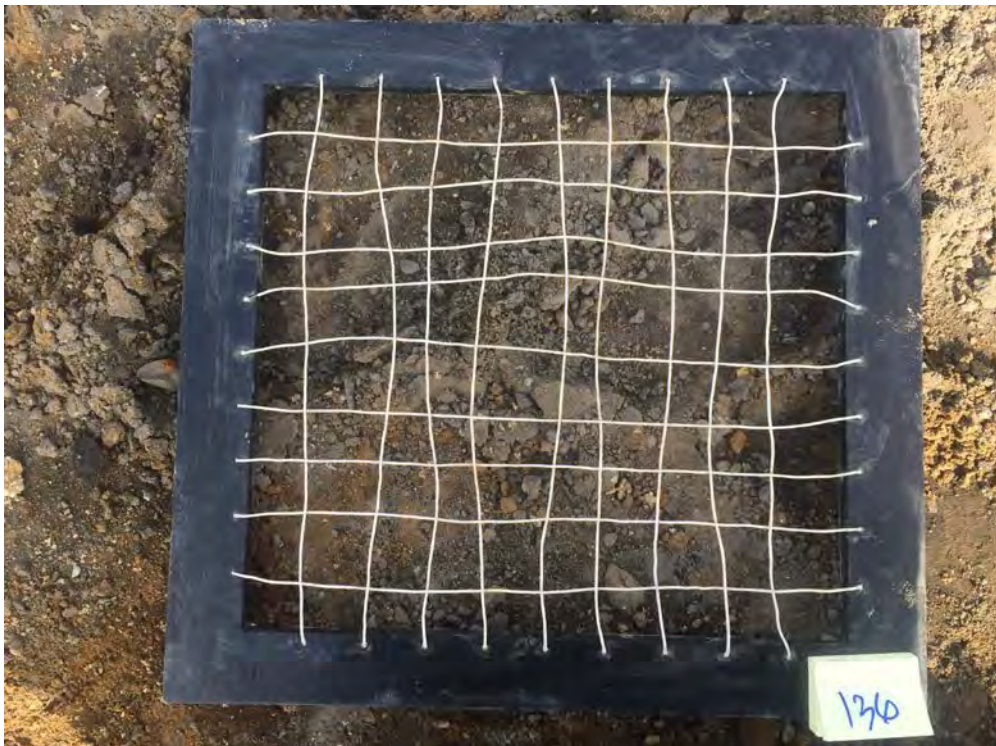
Variegated orange-brown silty medium sand with some gravel and sticks
