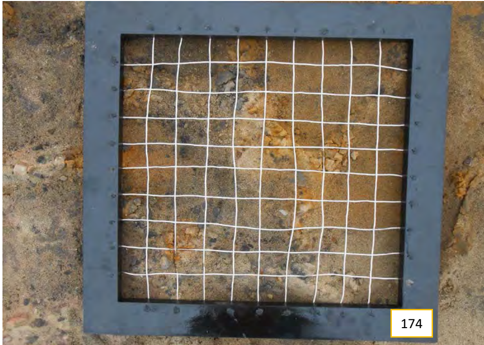
Variegated orange-brown silty fine sand with trace gravel and roots
