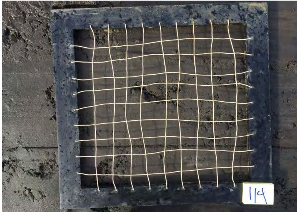
Dark brown silty fine sand with trace gravel
